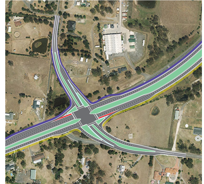
The Northern Road and Badgerys Creek Road intersection will be upgraded to include signalised traffic lights
