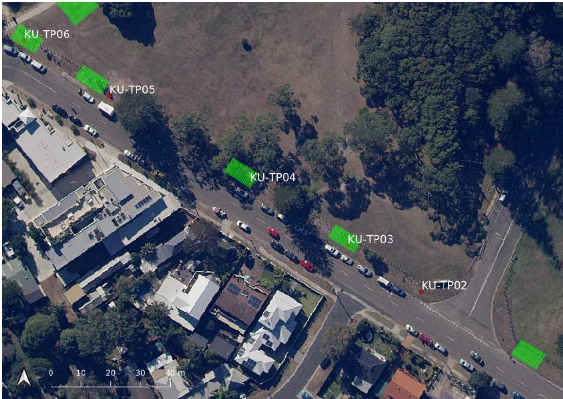
Figure 4.4: Kurnell study area, footpath. GPR survey lines are shown in green.
