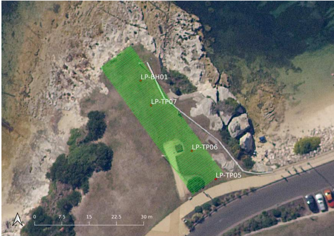
Figure 4.2: La Perouse study area, downslope. GPR survey lines are shown in green.
