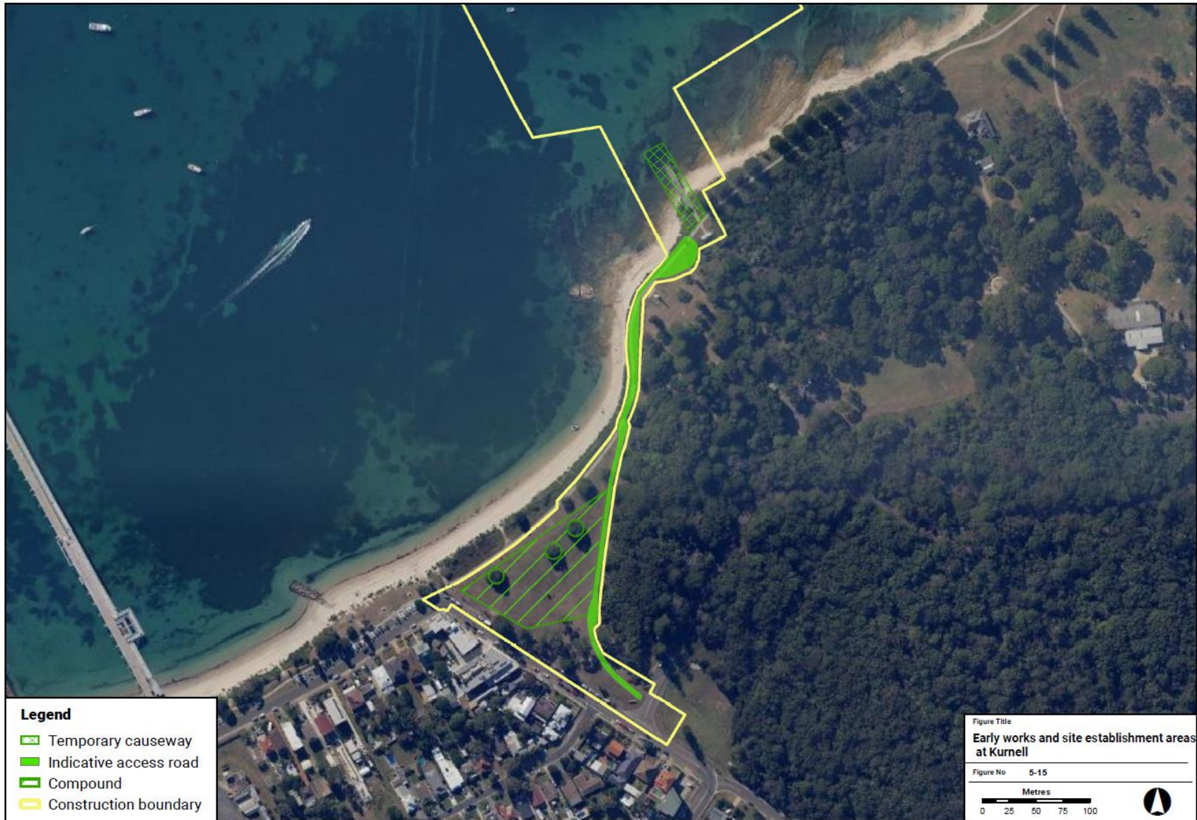
Figure 5-15: Early works and site establishment areas at Kurnell
