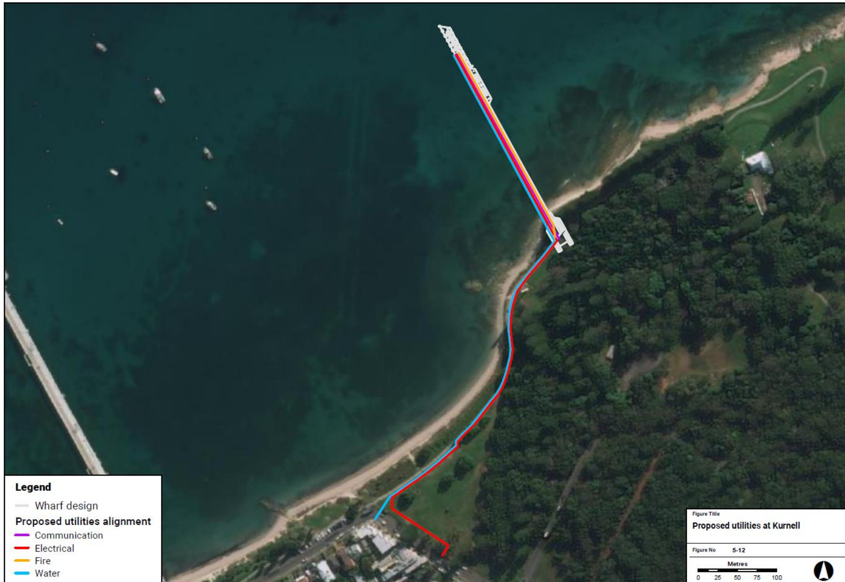
Figure 5-12: Proposed utilities at Kurnell
