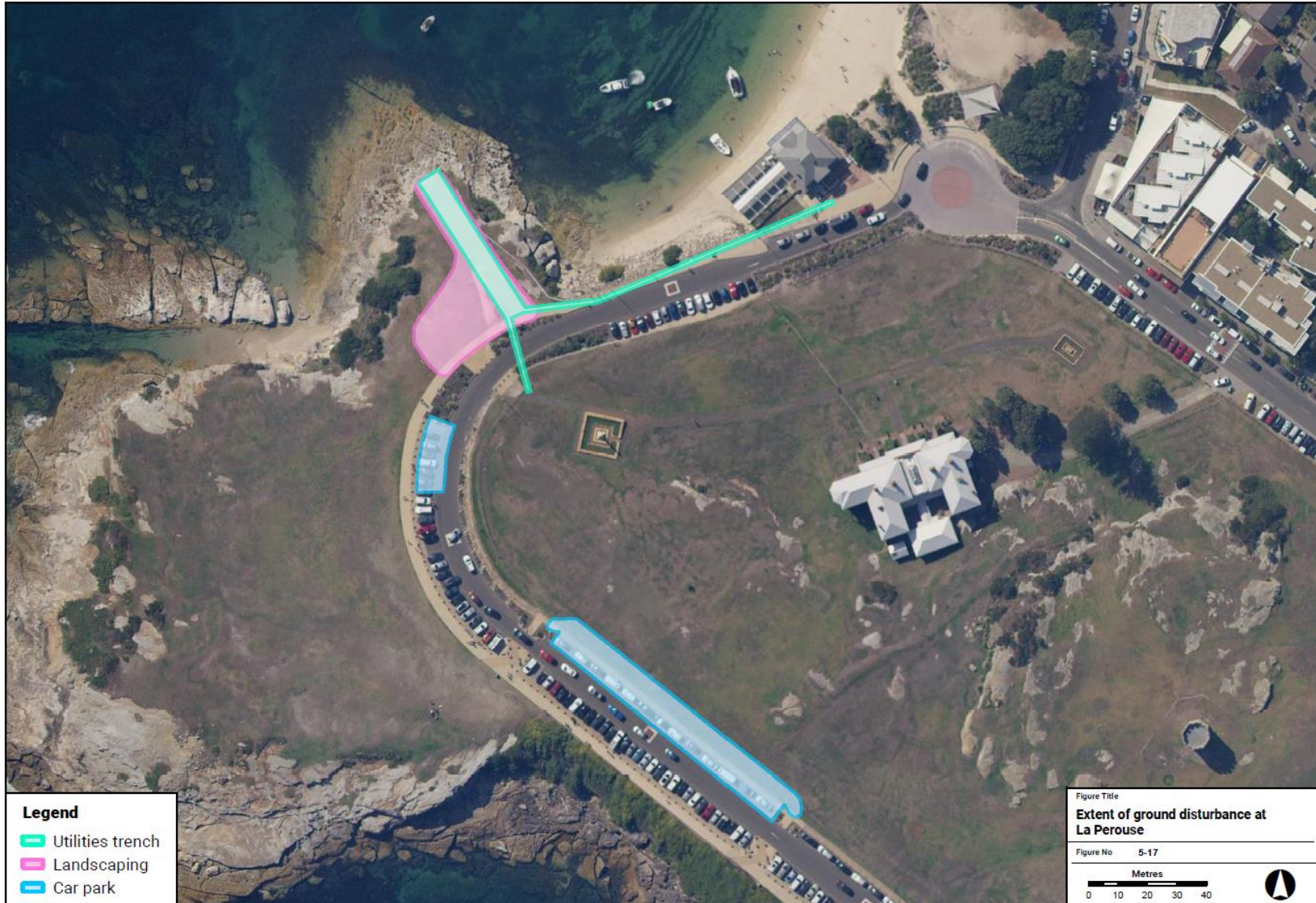
Figure 5-17: Extent of ground disturbance at La Perouse
