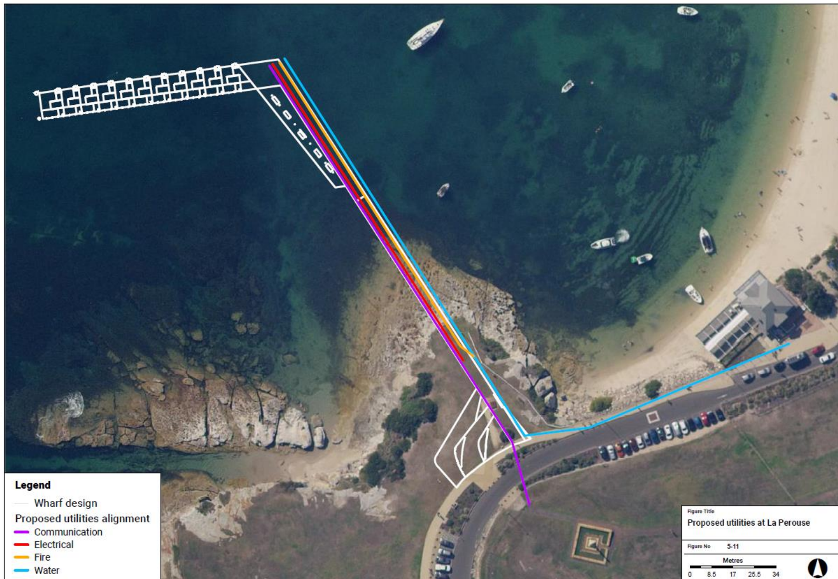
Figure 5-11: Proposed utilities at La Perouse
