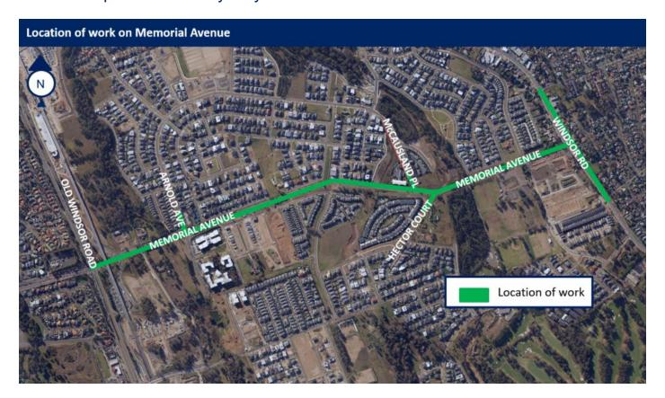
Transport for NSW is upgrading Memorial Avenue from a two lane to a four lane road with the option to expand to six lanes if needed in the future. This will improve traffic flow, ease congestion and reduce travel times along Memorial Avenue and nearby roads especially during the morning and afternoon peaks.
