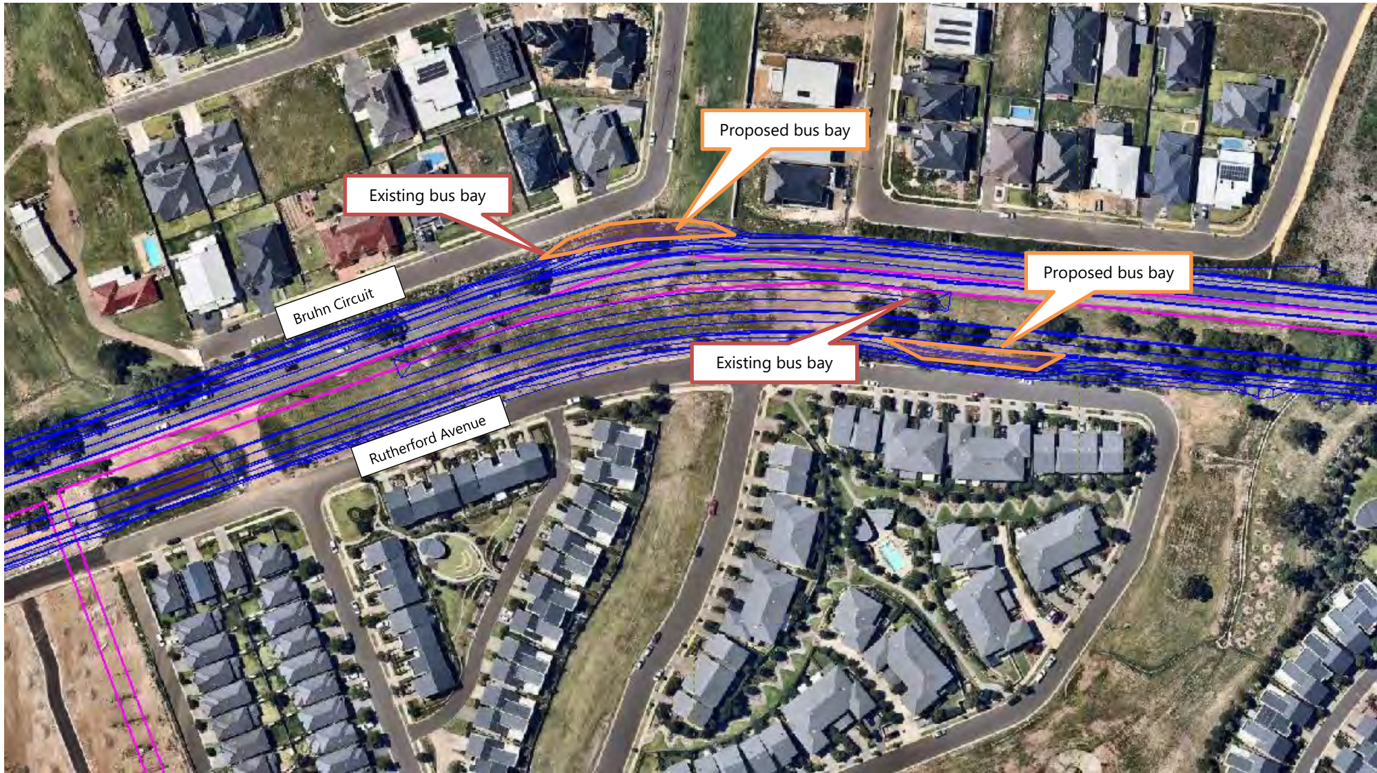
Figure 2 Existing and proposed bus bays
