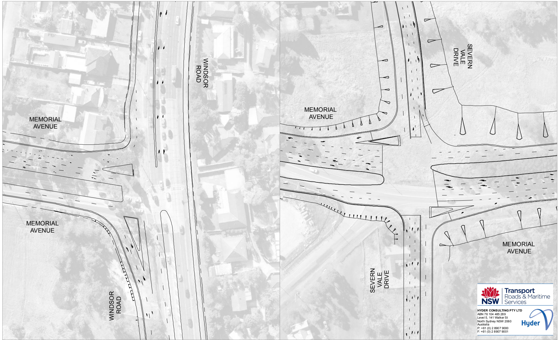
Figure 3-9: Proposed layout of Windsor Road / Memorial Avenue intersection and Memorial Avenue / Severn Vale Drive intersection
