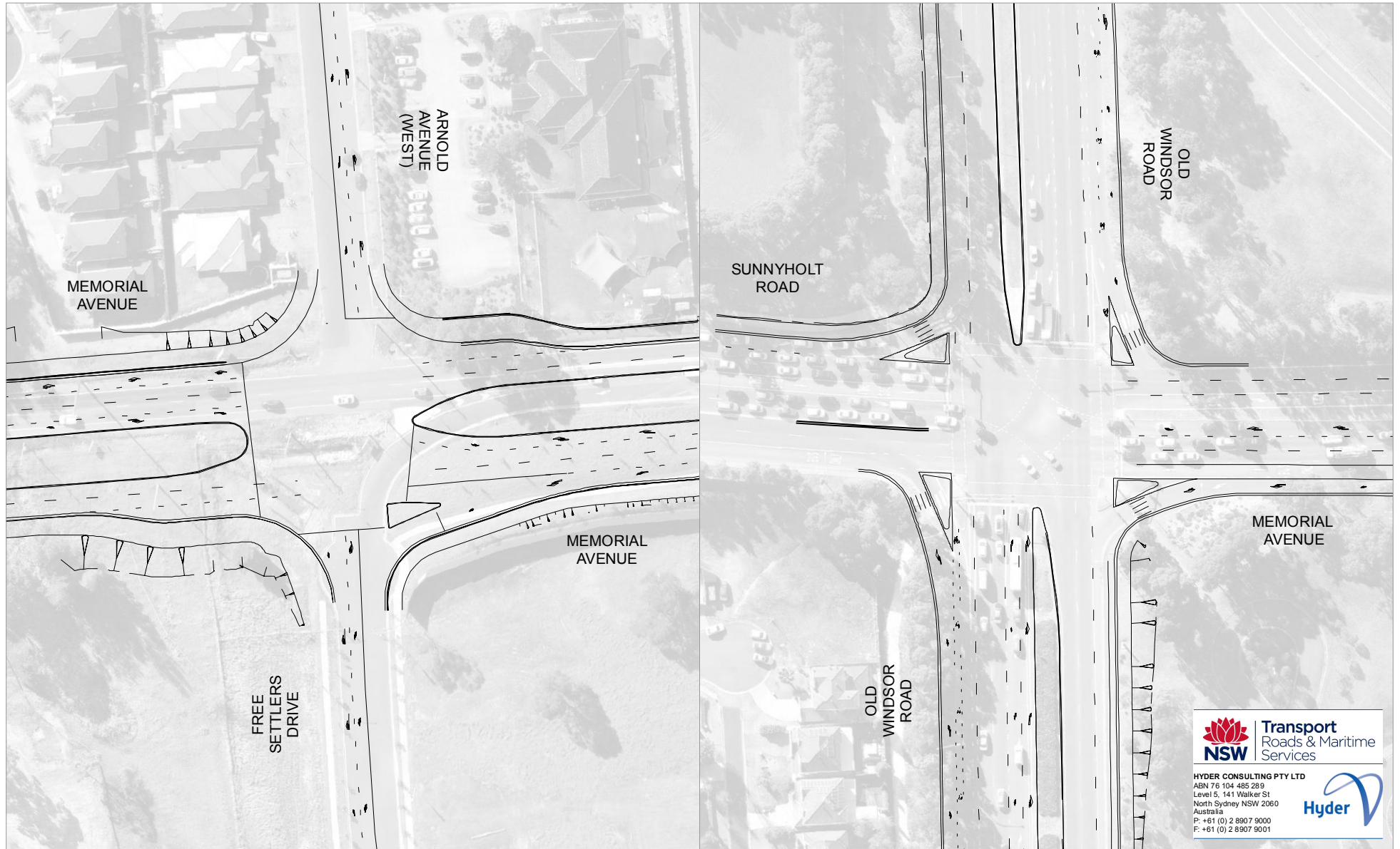
Figure 3-10: Proposed layout of Memorial Ave / Arnold Ave (W) / Free Settlers Dr intersection & Old Windsor Rd / Memorial Ave/ Sunnyholt Rd intersection
