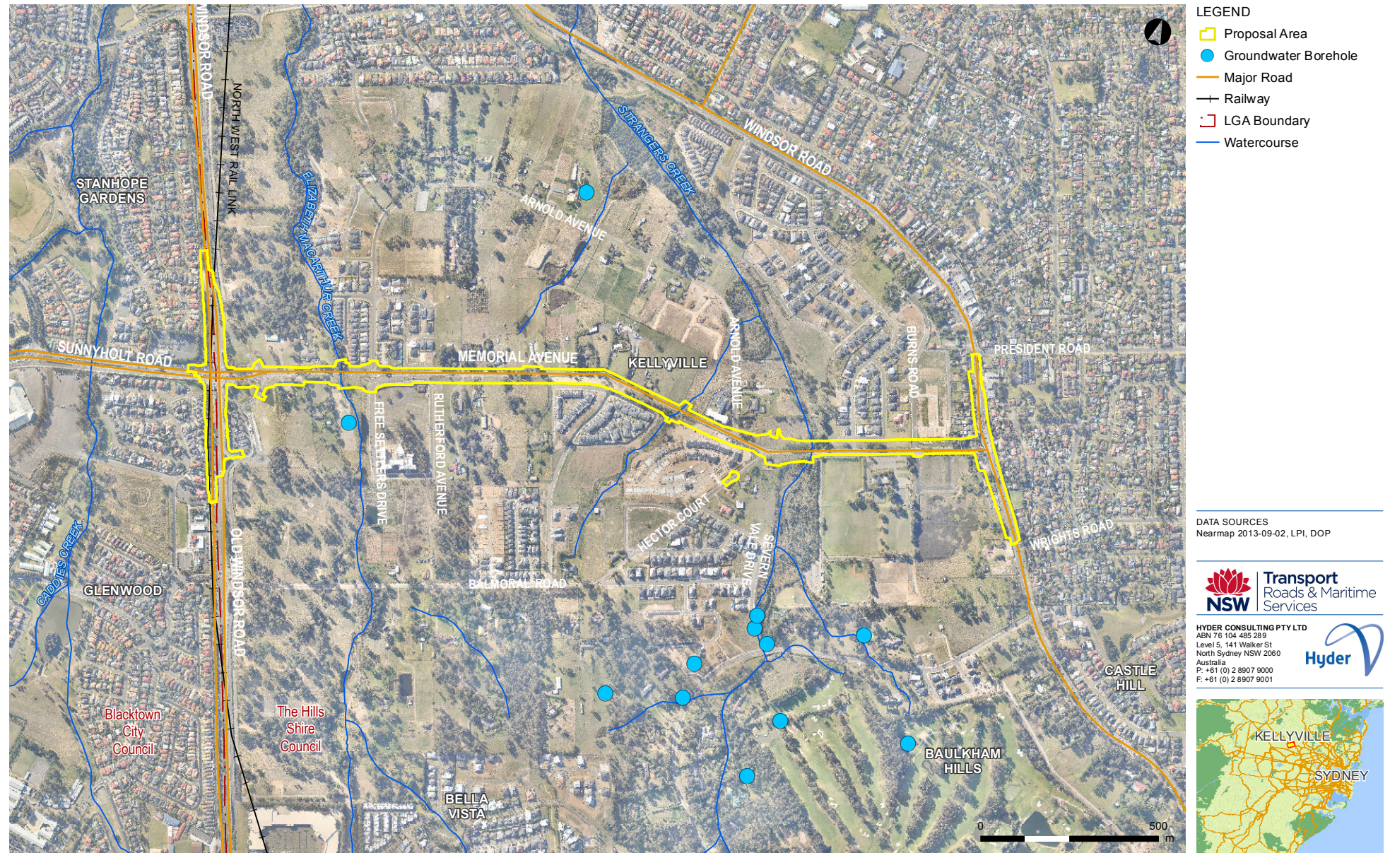
Figure 6-3: Indicative location of groundwater boreholes within 2 kilometres of the proposal area (Source: NSW Natural Resource Atlas 2014)
