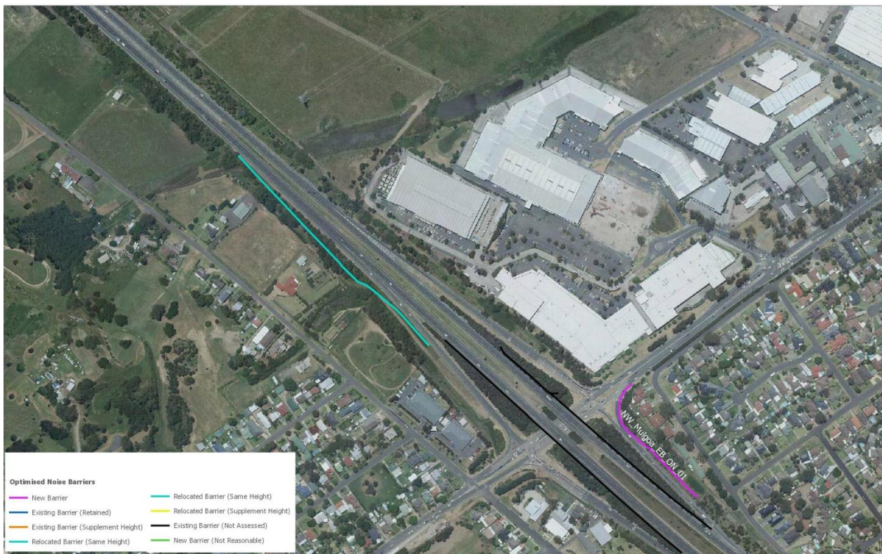
Figure 27 Mulgoa Road interchange - recommended noise barrier
