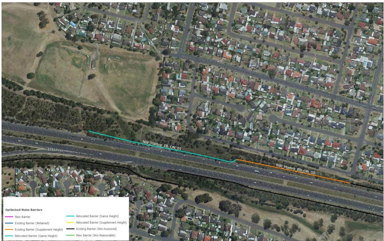
Figure 22 Mamre Road interchange - recommended noise barrier
