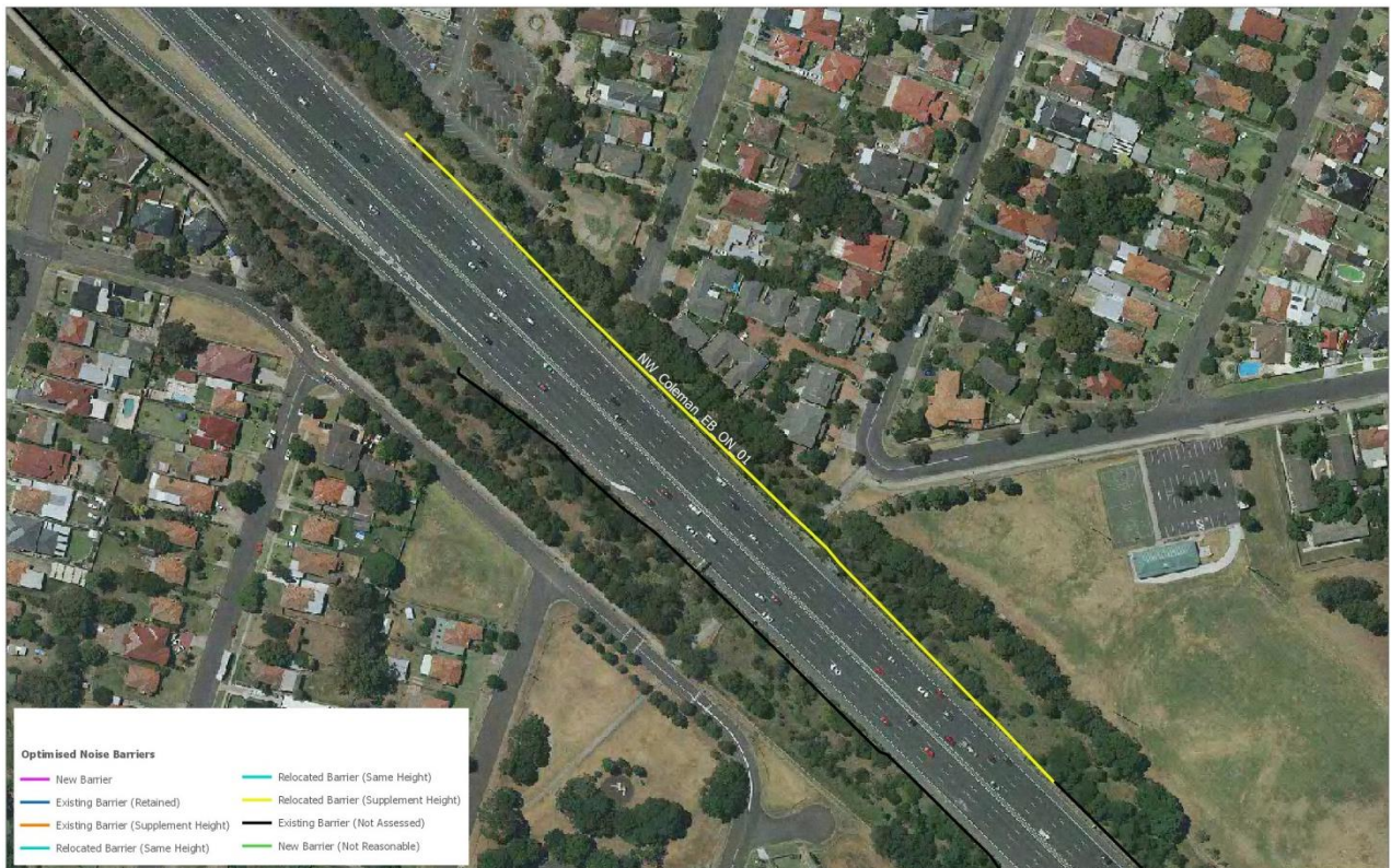
Figure 7 Coleman Street interchange - recommended noise barrier
