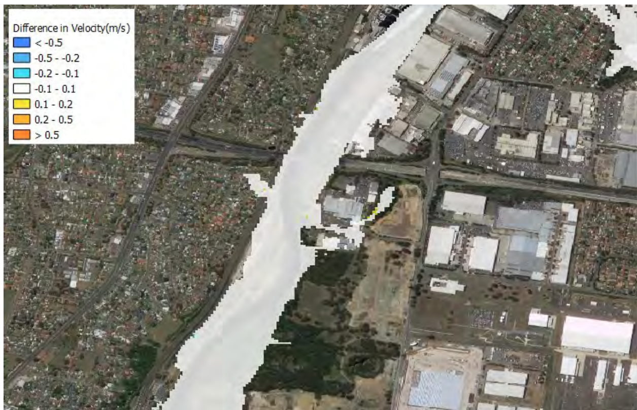
Figure 7-6 Predicted changes in peak flow velocities as a result of proposal – 1% AEP
