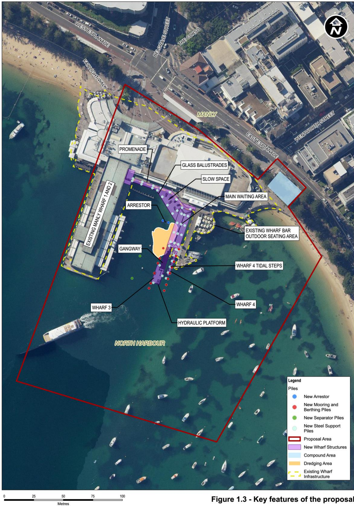
Figure 28 Plan showing the project boundary and an overlay of the new proposal over the existing Wharf. (Source: TfNSW, 2022)
