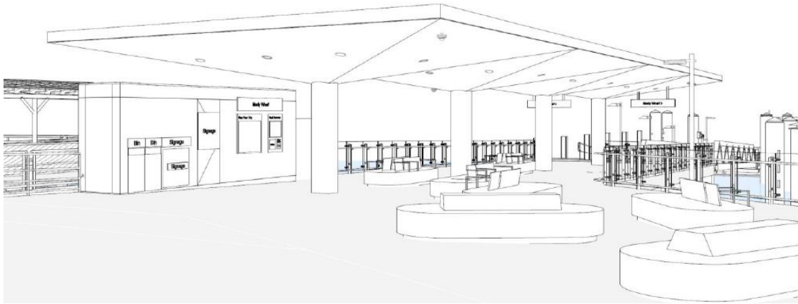
Figure 3.5 Concept design view of main waiting area, roof canopy, service pod, balustrades, screens and benches
