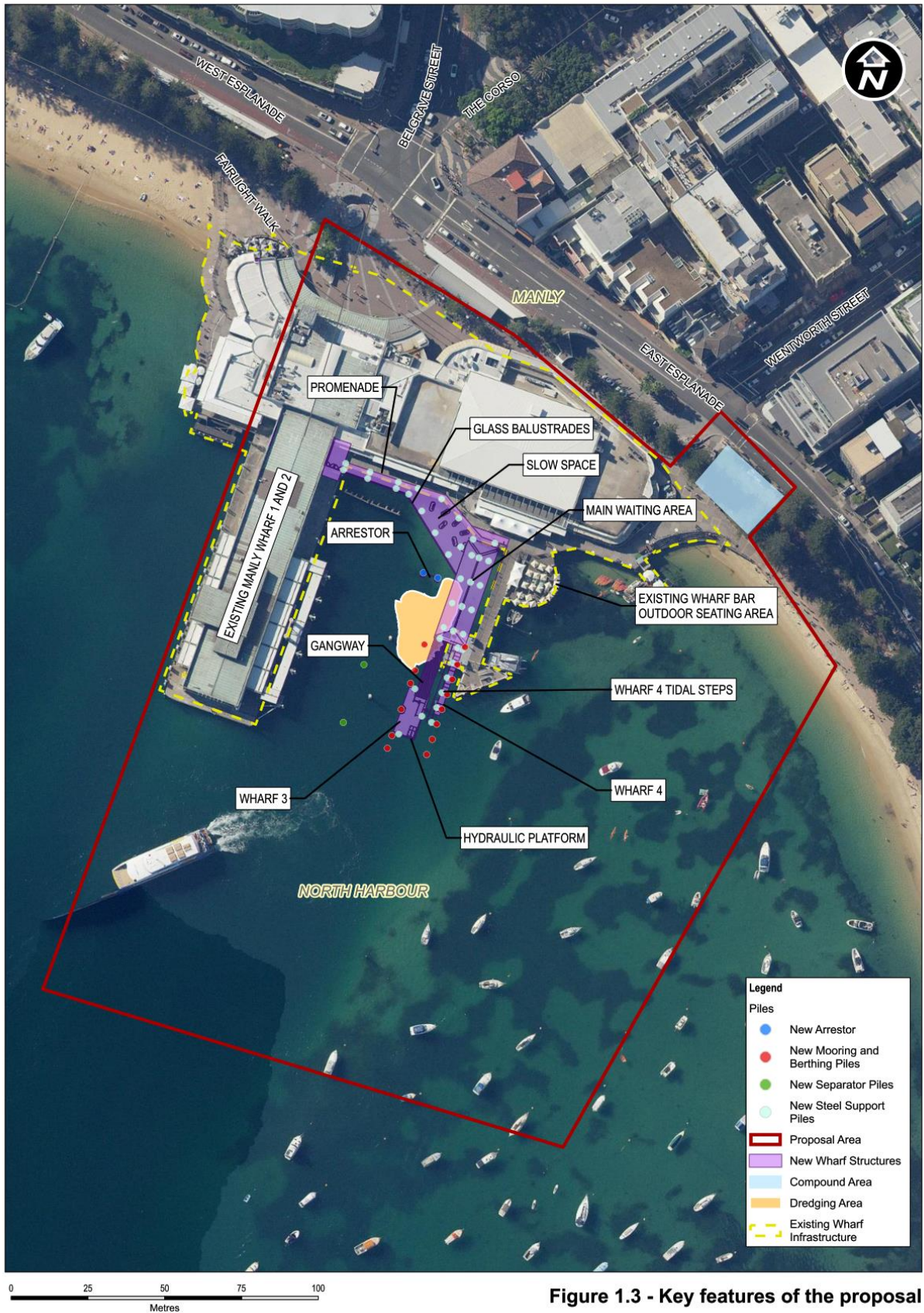
Figure 57 Plan showing the project boundary and an overlay of the new proposal over the existing Wharf. (Source: TfNSW, 2022)
