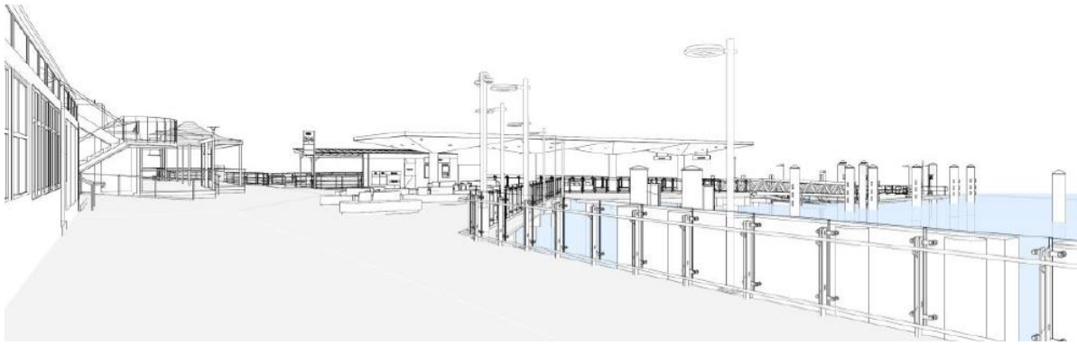
Figure 3.7 Sketch of concept design of the widened boardwalk, informal seating, and new light poles
