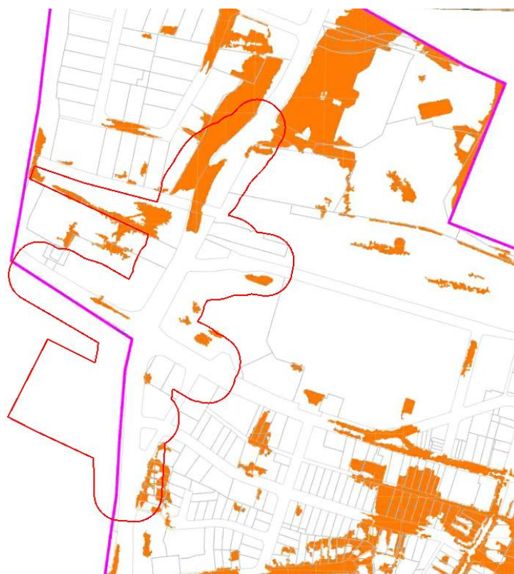
Figure 6: Mapping of areas affected by the 100 year Average Recurrence Interval (ARI), with the study area outlined in red (Cardno July 2015).
