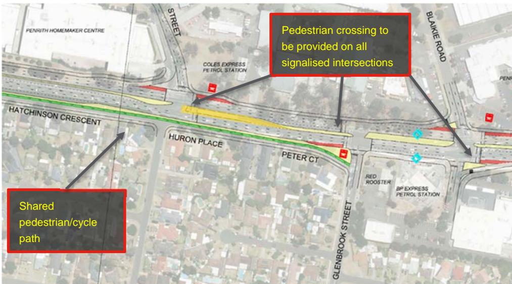
Figure 6-2 Pedestrian/Cycle Access Provided along Mulgoa Road between M4 and Blaikie Road
