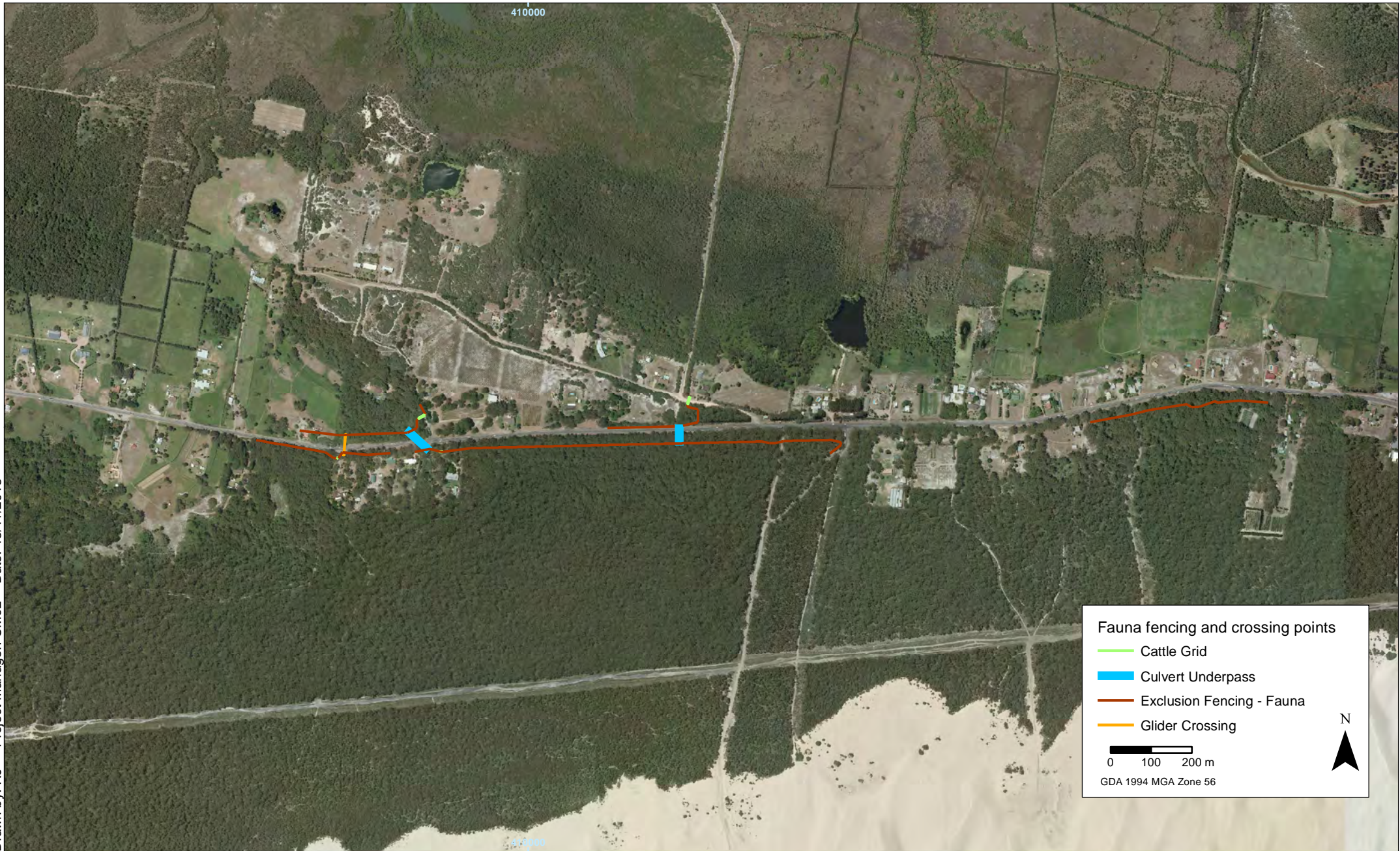
Location of fauna fencing and fauna crossing points Nelson Bay Road EPBC Referral Supplementary Information
