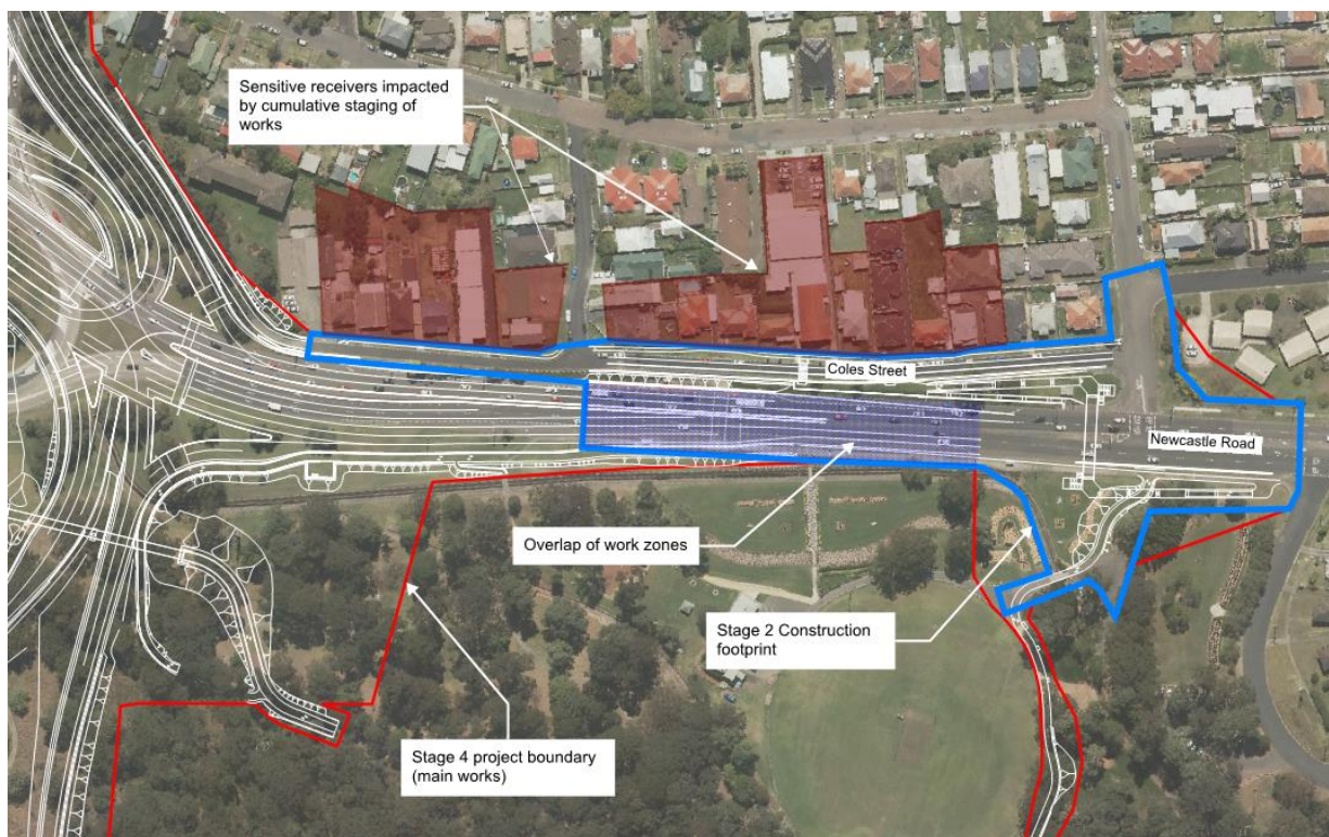
Figure 4.1: Cumulative impacts of RP2J construction on Newcastle Road
