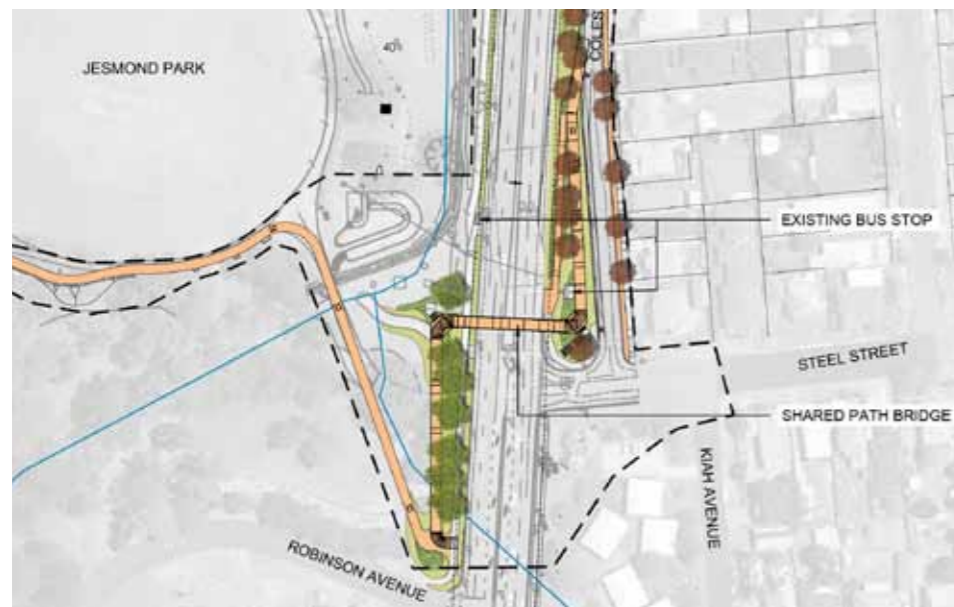
Figure 5.32 Plan illustrating the location of the proposed shared path bridge over Newcastle Road.
