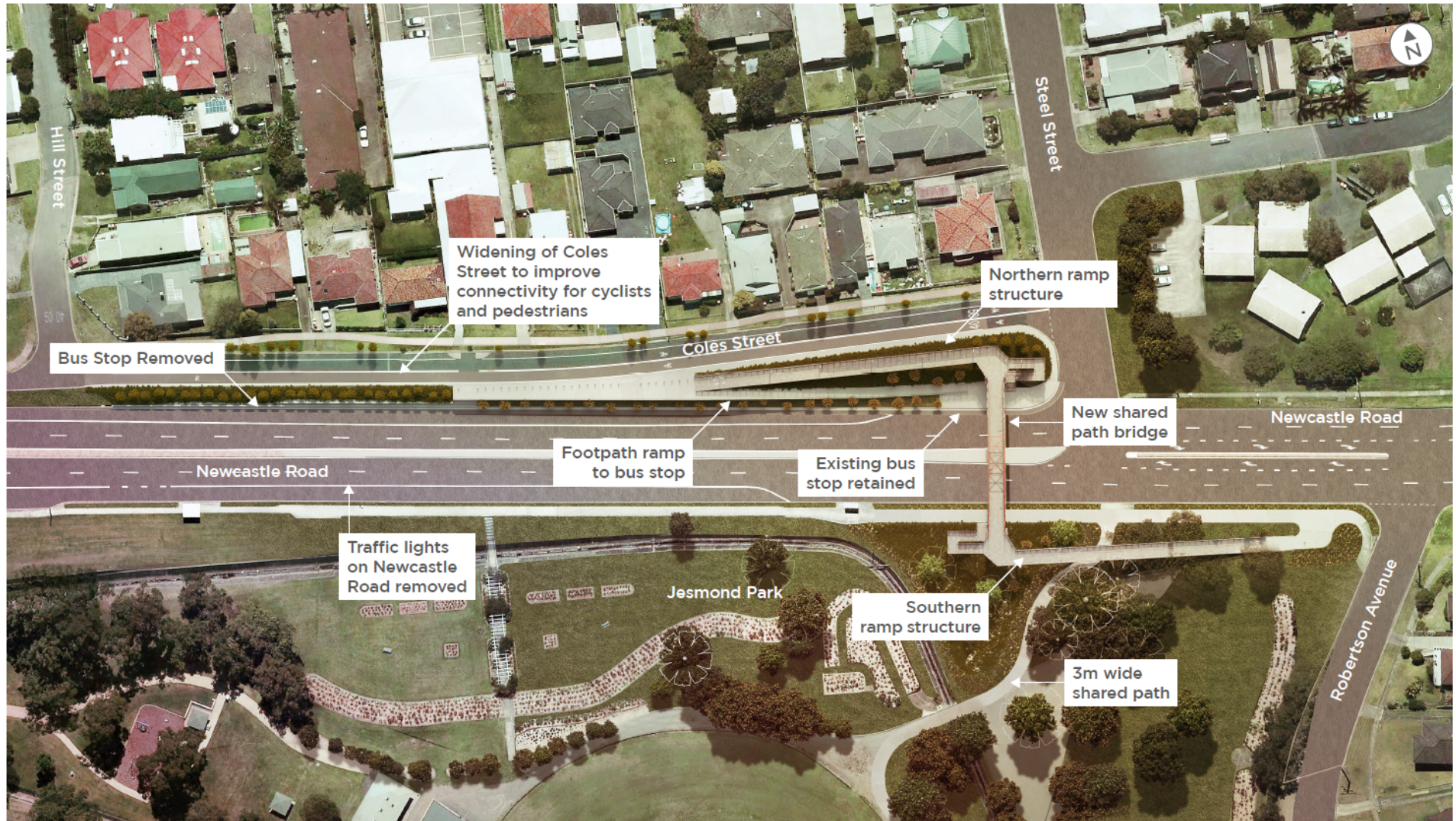
Figure 2-2: Shared Path Bridge (Bridge 7) works
