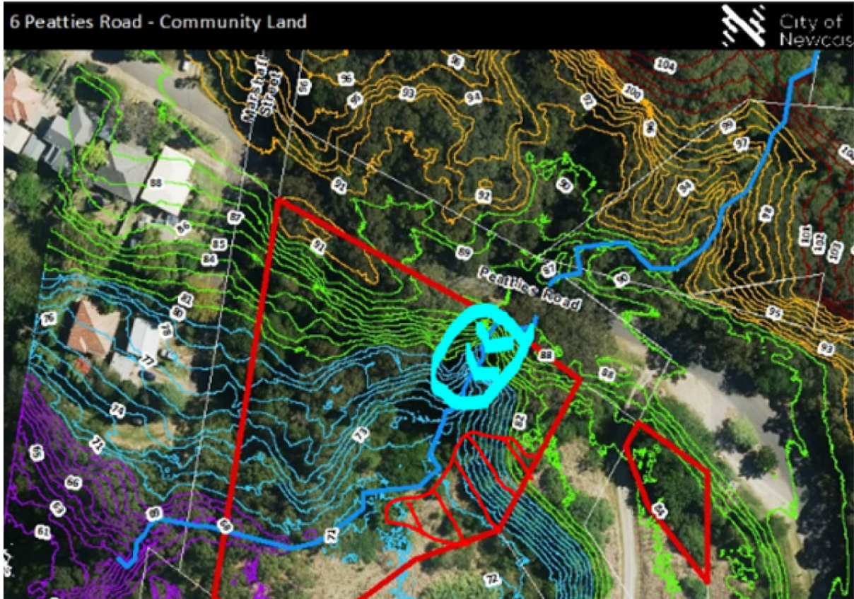
Figure 3 – Indicative drainage line protection area (in light blue) downstream of the Peatties Road culvert ( Condition E89 )
