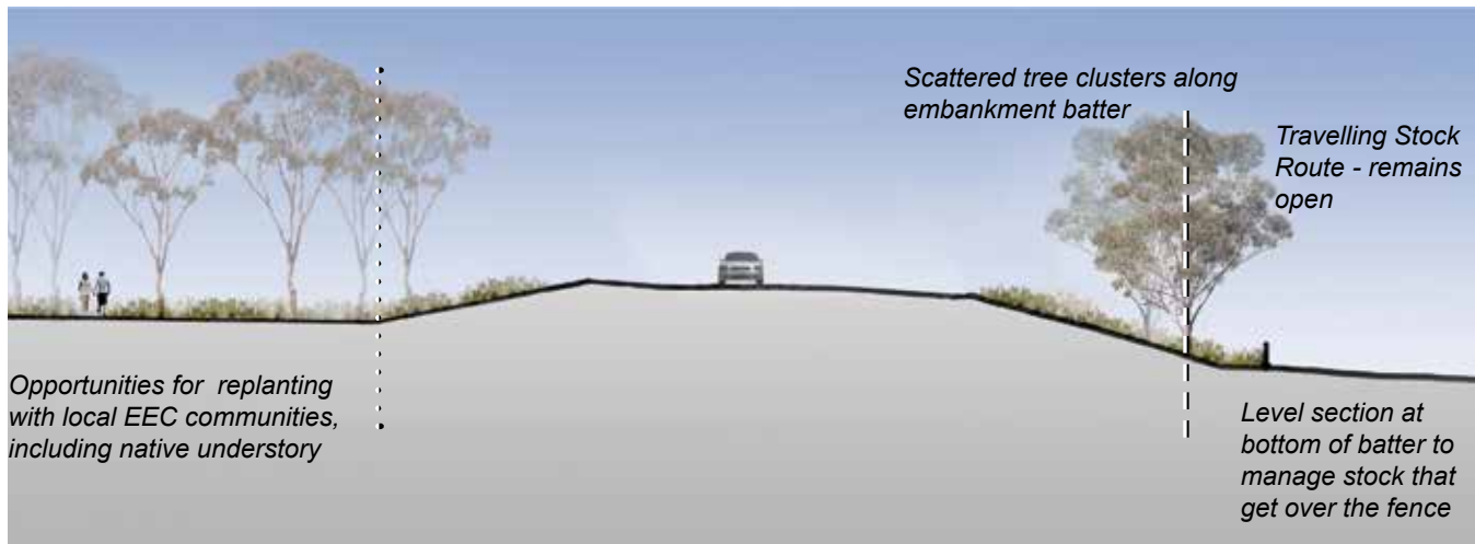
Figure 87 Travelling Stock Route section - in fill batter
