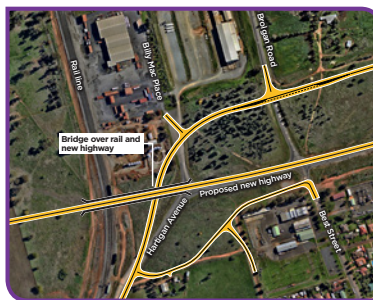
Inset detail: Bridge over Hartigan Avenue and the Broken Hill and Parkes to Narromine rail lines
