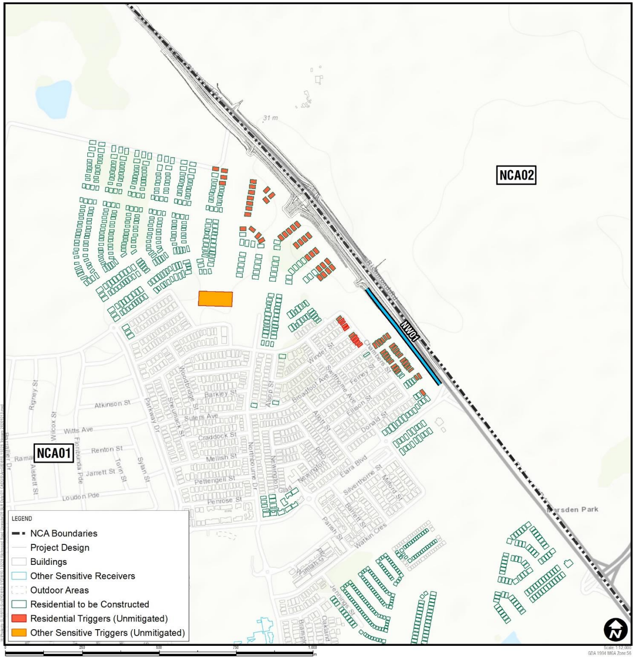
Figure 20 Indicative Noise Barriers Considered for Further Investigation
