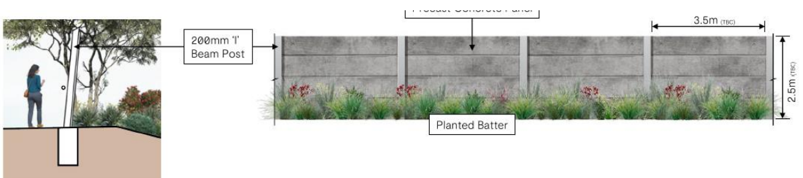
Figure 5.9 Concrete panel noise wall
