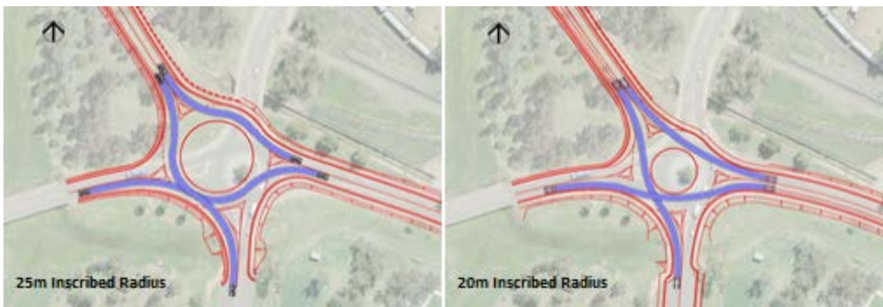
Figure 8.3: Vehicle paths and relative deflections for R20 metres and R25 metre roundabouts
