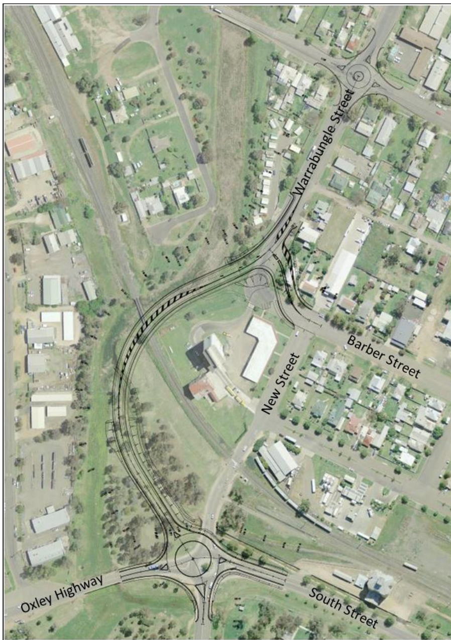
Figure 3.1: Gunnedah second road over rail bridge
