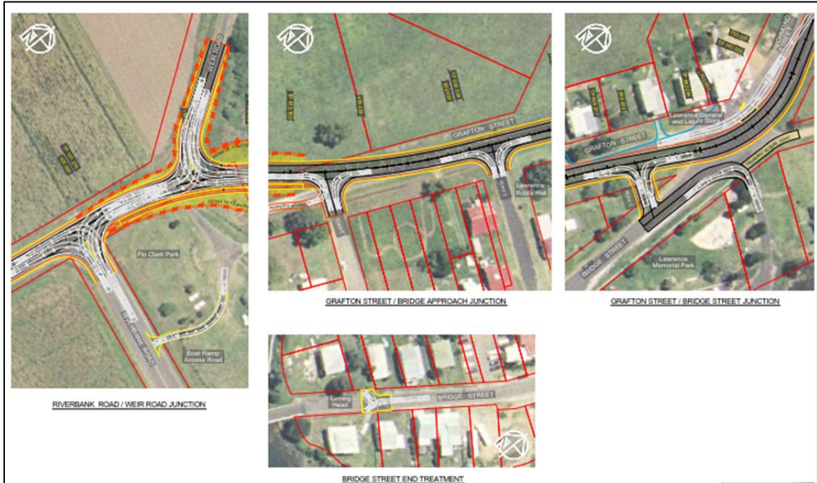
Figure 8.3 Proposed intersection treatments for preferred option showing turning paths
