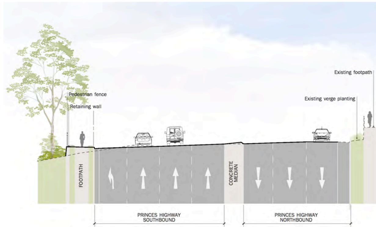
Figure 44. Section 1 through the Princes Highway - Chainage 76780 (Scale 1:250)
