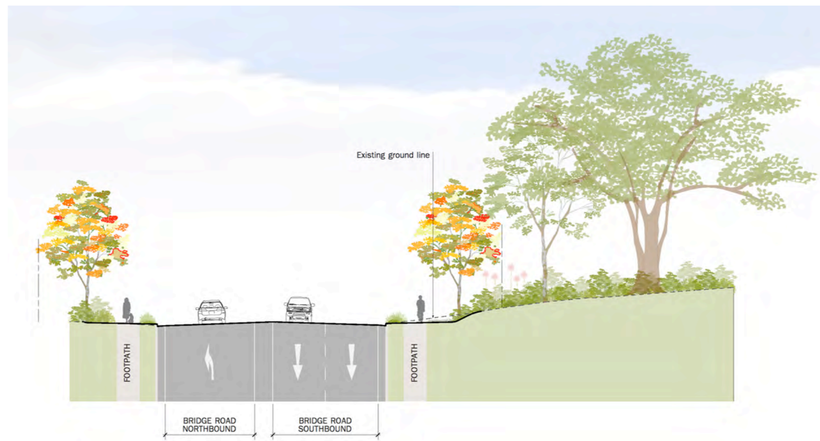
Figure 63. Section 8 through the Bridge Road - Chainage 80 (Scale 1:250)
