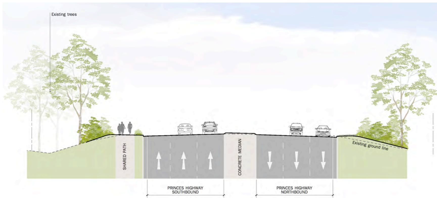
Figure 60. Section 7 through the Princes Highway - Chainage 78080 (Scale 1:250) Note: 1. Proposed planting shown at maturity 2. Subject to further design development and consultation.
