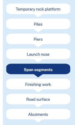
The new Nowra Bridge is being built using a specialised technique known as incremental launching. There will be 19 bridge deck segments in total for the new bridge.
