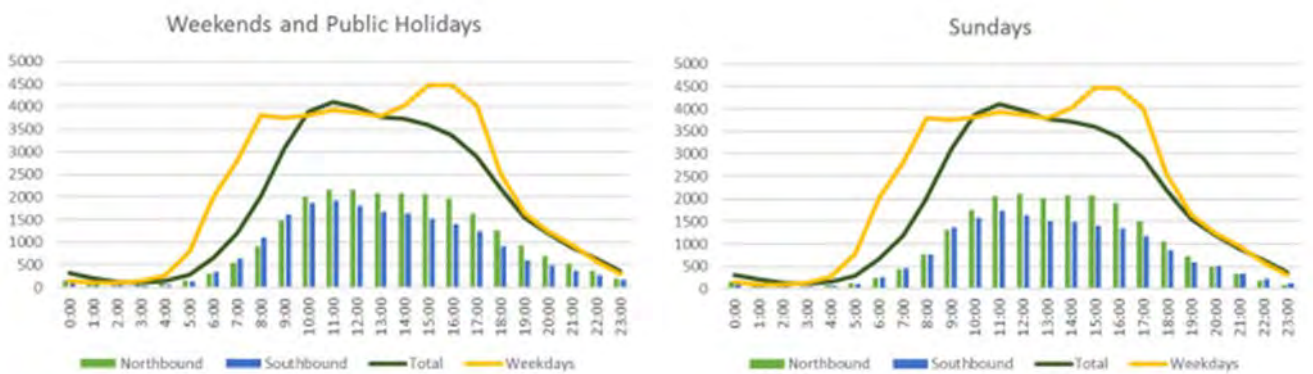
Figure 3-7: Princes Highway Average Hourly Traffic Volume on Weekends and Public Holidays (left) and Sundays (right) for 2017
