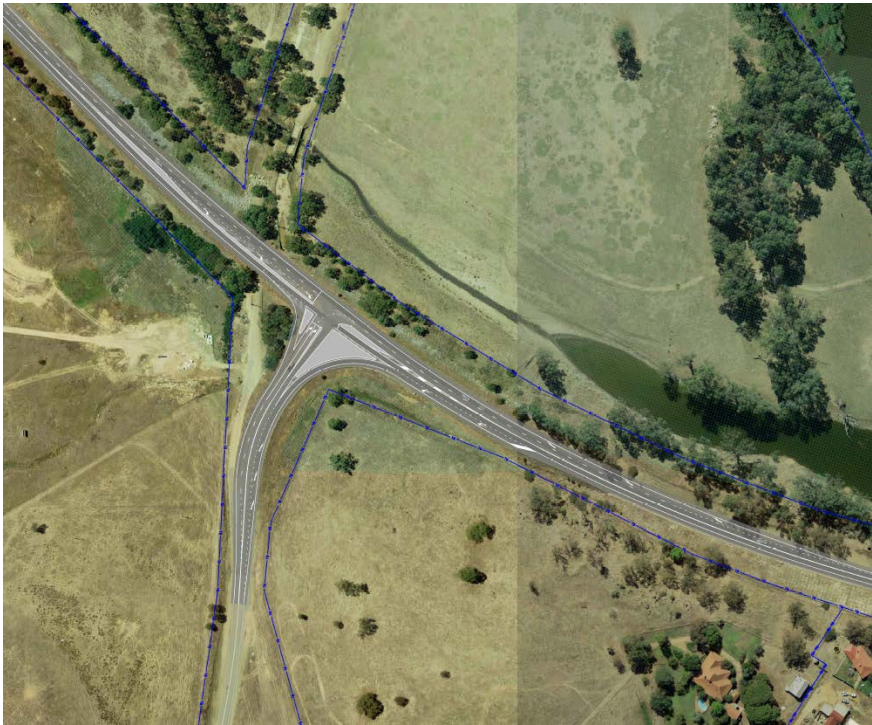
Figure 2 Proposed Old Narrandera Road intersection upgrade – strategic design only, subject to change
