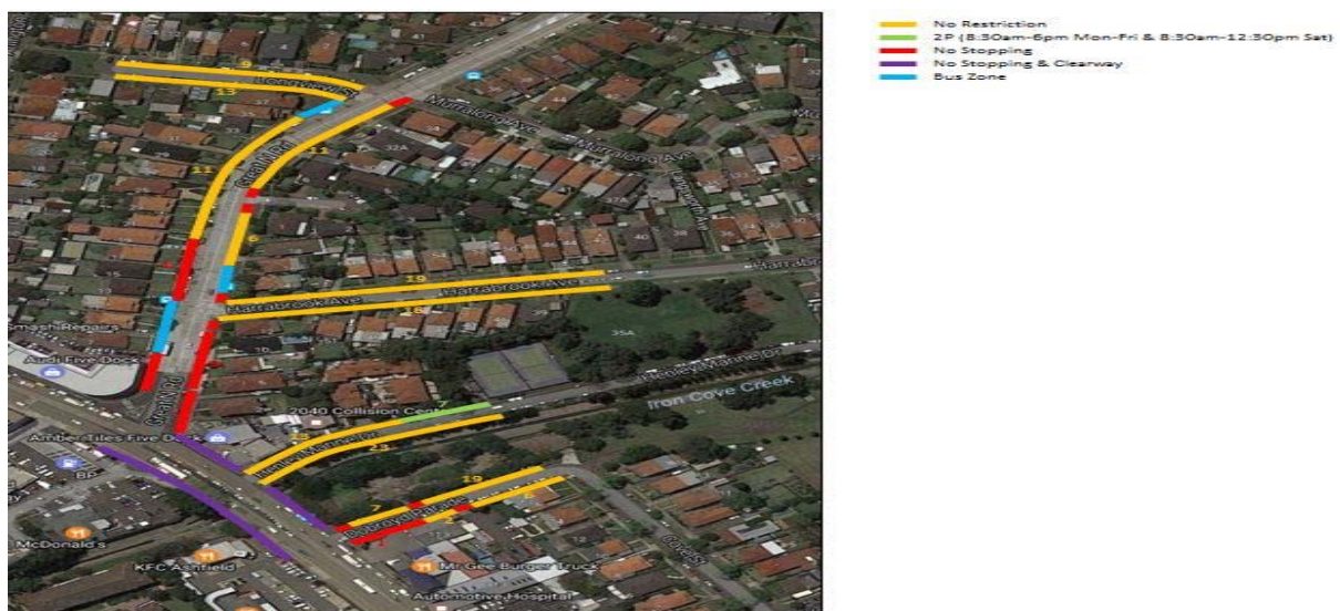
Figure 3: Parking Inventory at Completion of Works
