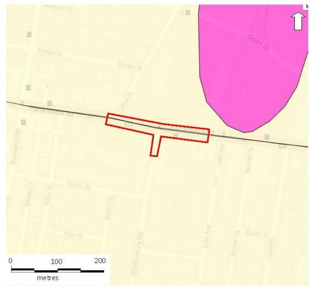
Figure 6-8: Acid sulfate soils in vicinity of the proposal. Red line indicates the proposal area. peach shading indicates class 5 ASS; bright pink shading indicates class 2 ASS (Source: DP&E planning viewer 2015)
