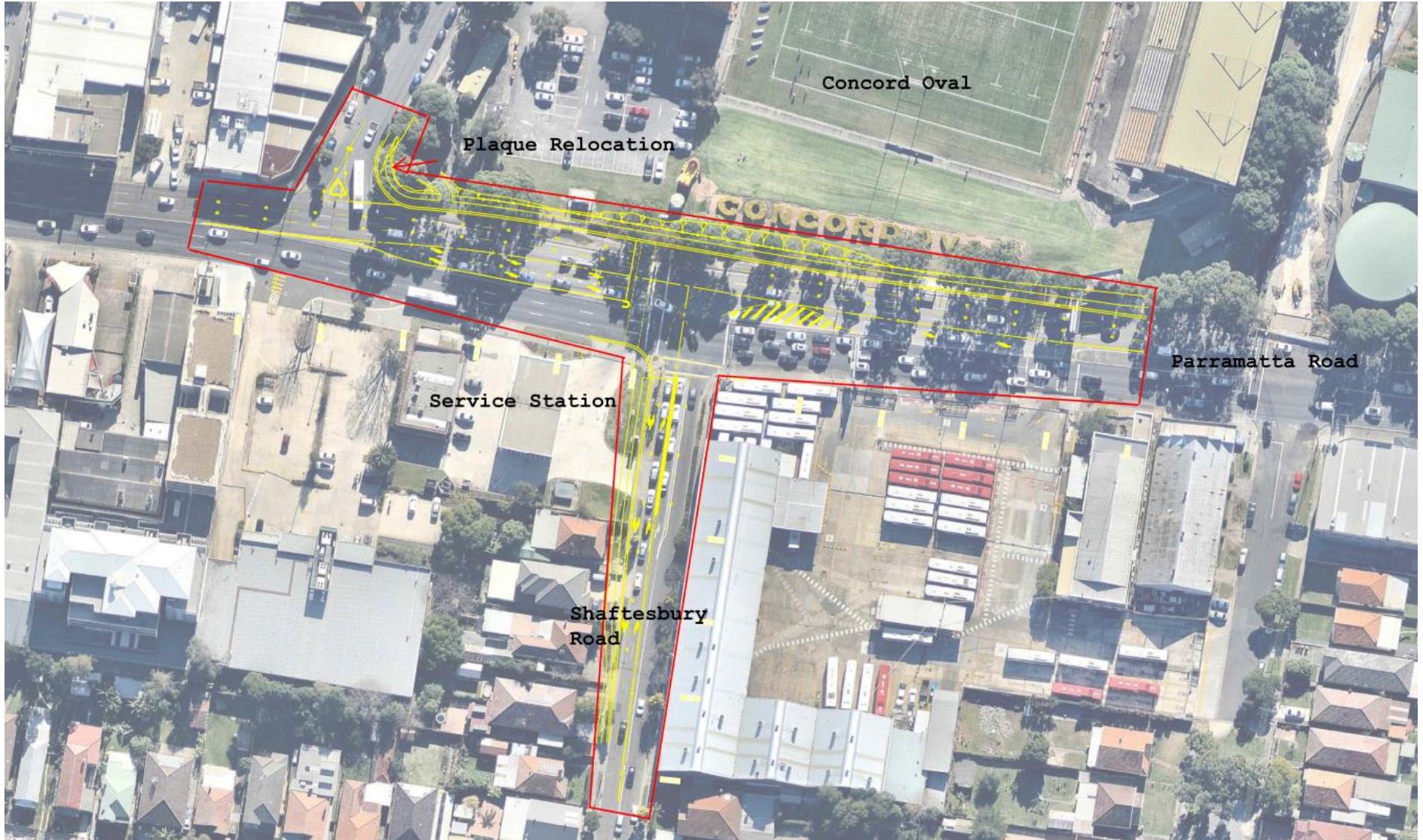
Figure 1-2 Design of the proposed Parramatta Road & Shaftesbury Road intersection upgrade. The proposal area boundary is shown in red.
