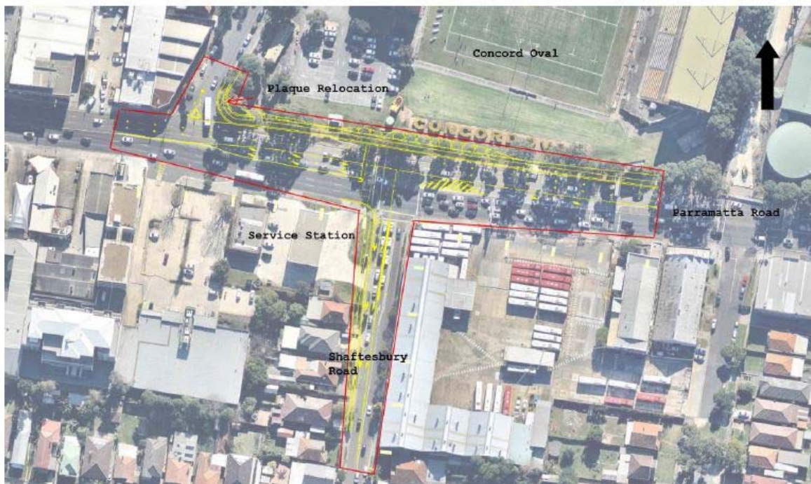
Figure 1-2 Design of the proposed Parramatta Road & Shaftesbury Road intersection upgrade. The proposal area boundary is shown in red.
