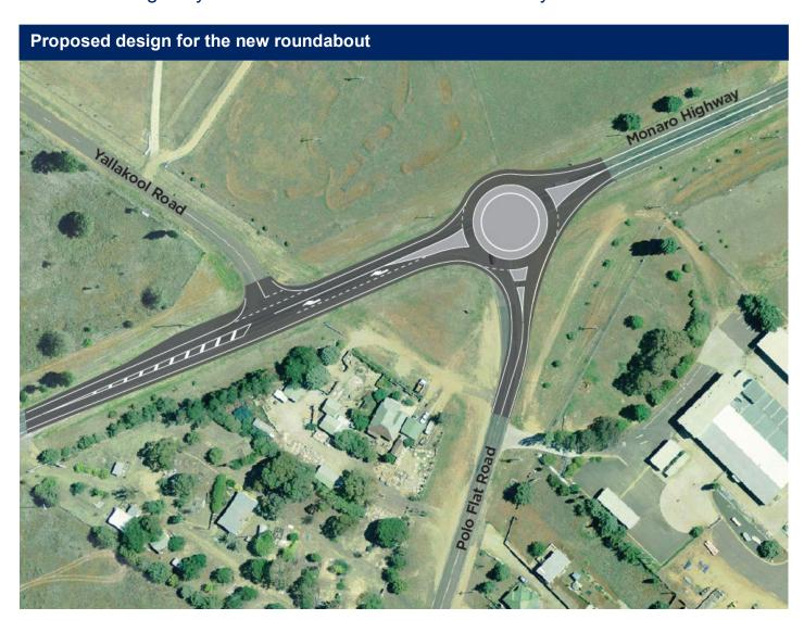
Polo Flat Road provides access to Cooma's industrial area and carries a high number of heavy vehicles. The proposed roundabout will deliver safer journeys for light and heavy vehicles sharing the road. A dedicated right turn lane for motorists turning into Yallakool Road will also be built as part of this upgrade.
