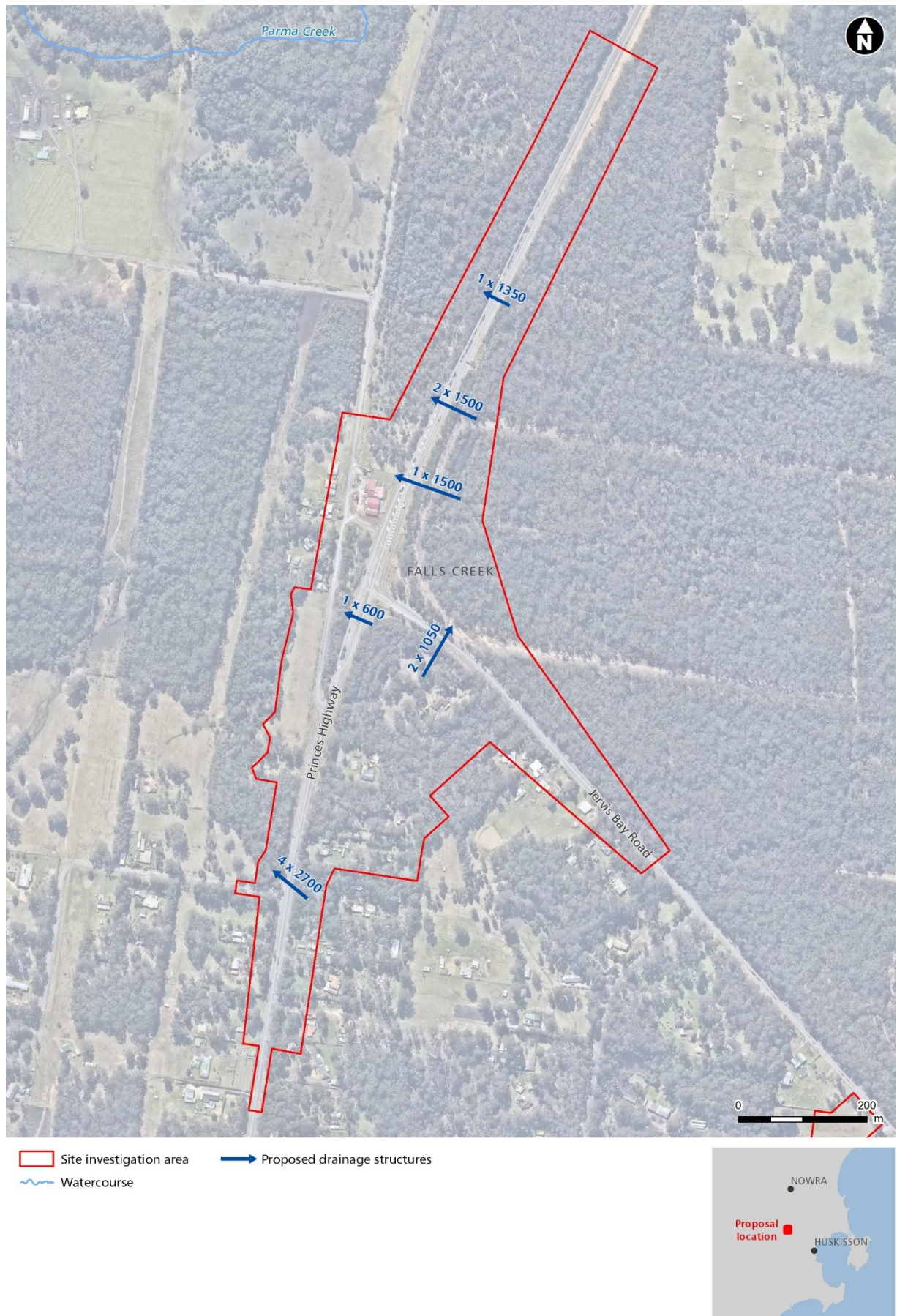
Figure 14 Overview of proposed drainage features for the design proposal
