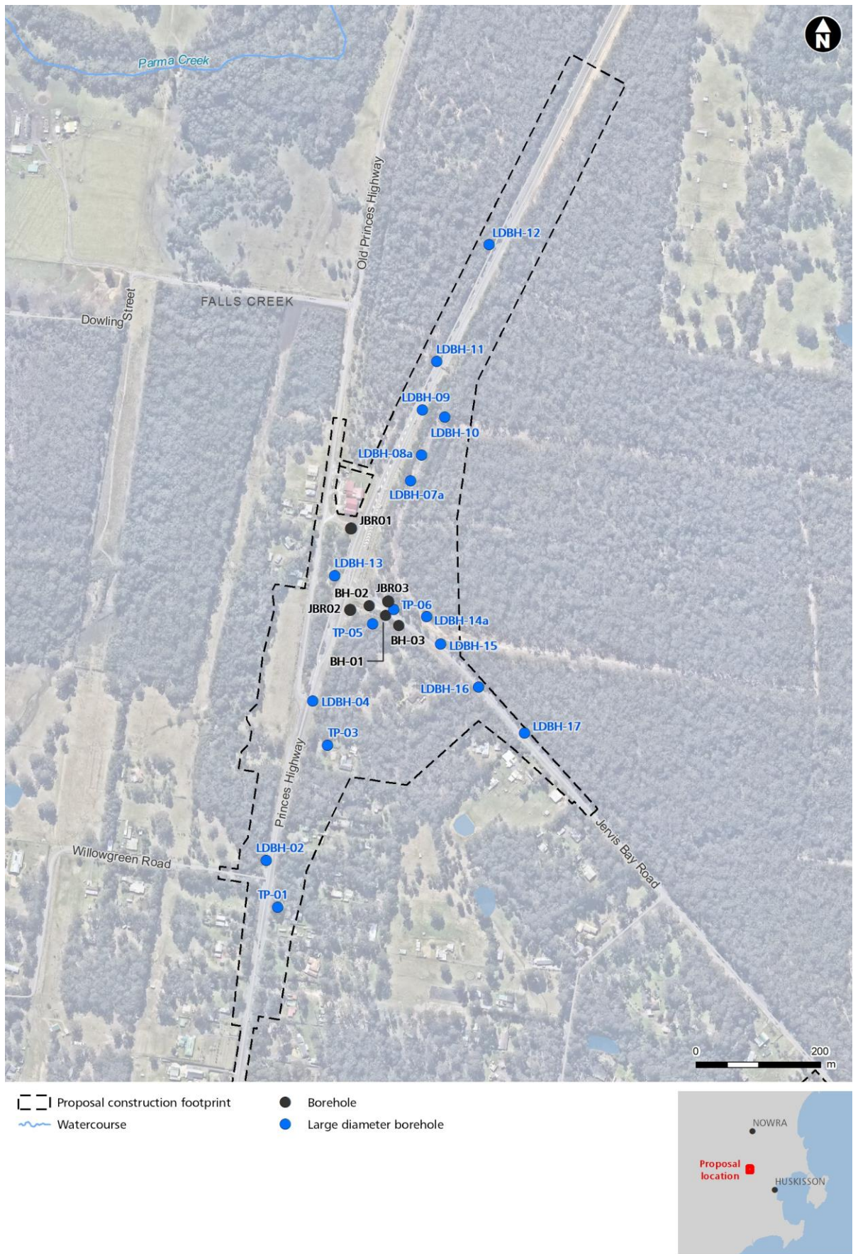
Figure 6-27 Geotechnical investigations borehole locations
