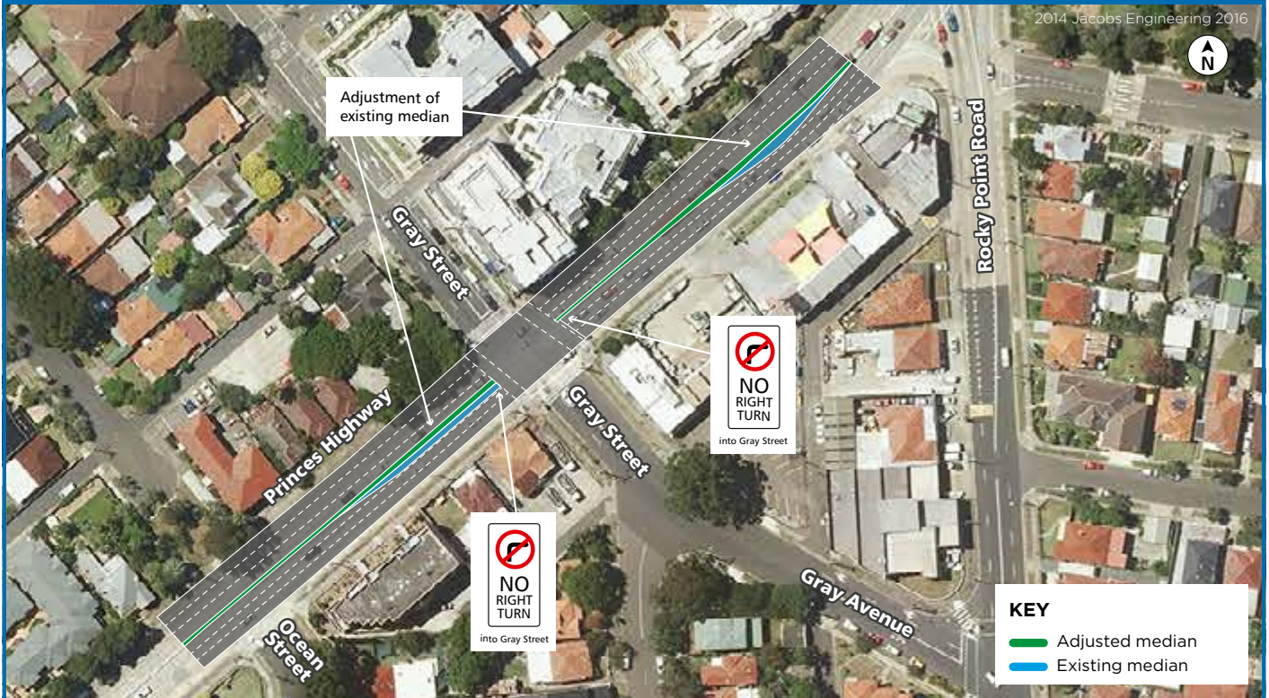
Improvements at the intersections of Princes Highway, Rocky Point Road and Gray Street, Kogarah.
