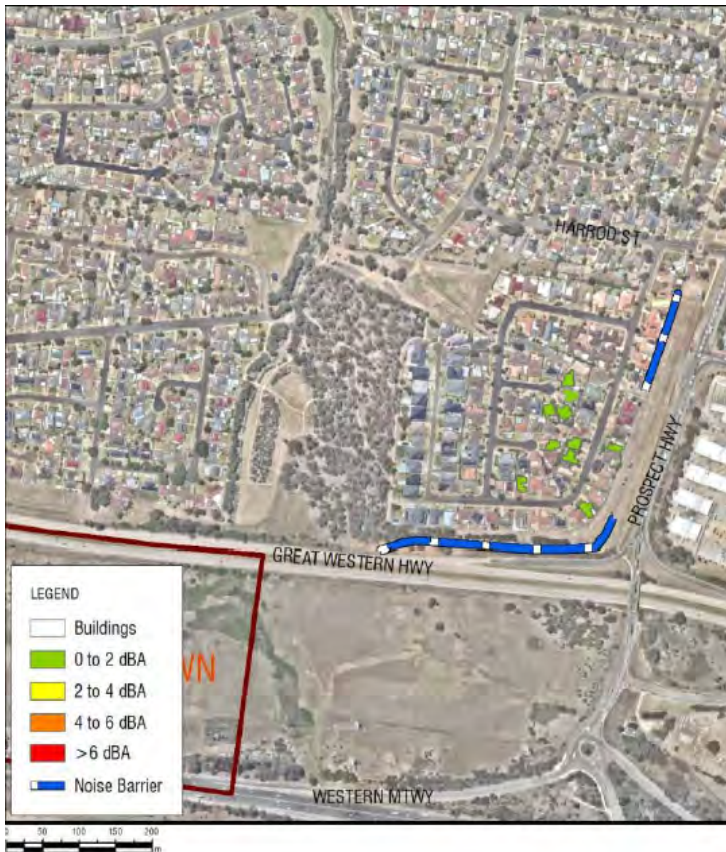
Figure 6.2 Predicted noise levels as a result of the changes to noise wall NW_NB01
