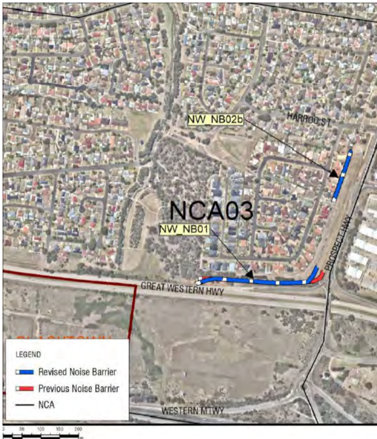
Figure 6-1 Alignment of original Detailed Design noise wall NW_NB01 (red) and new proposed alignment (blue)
