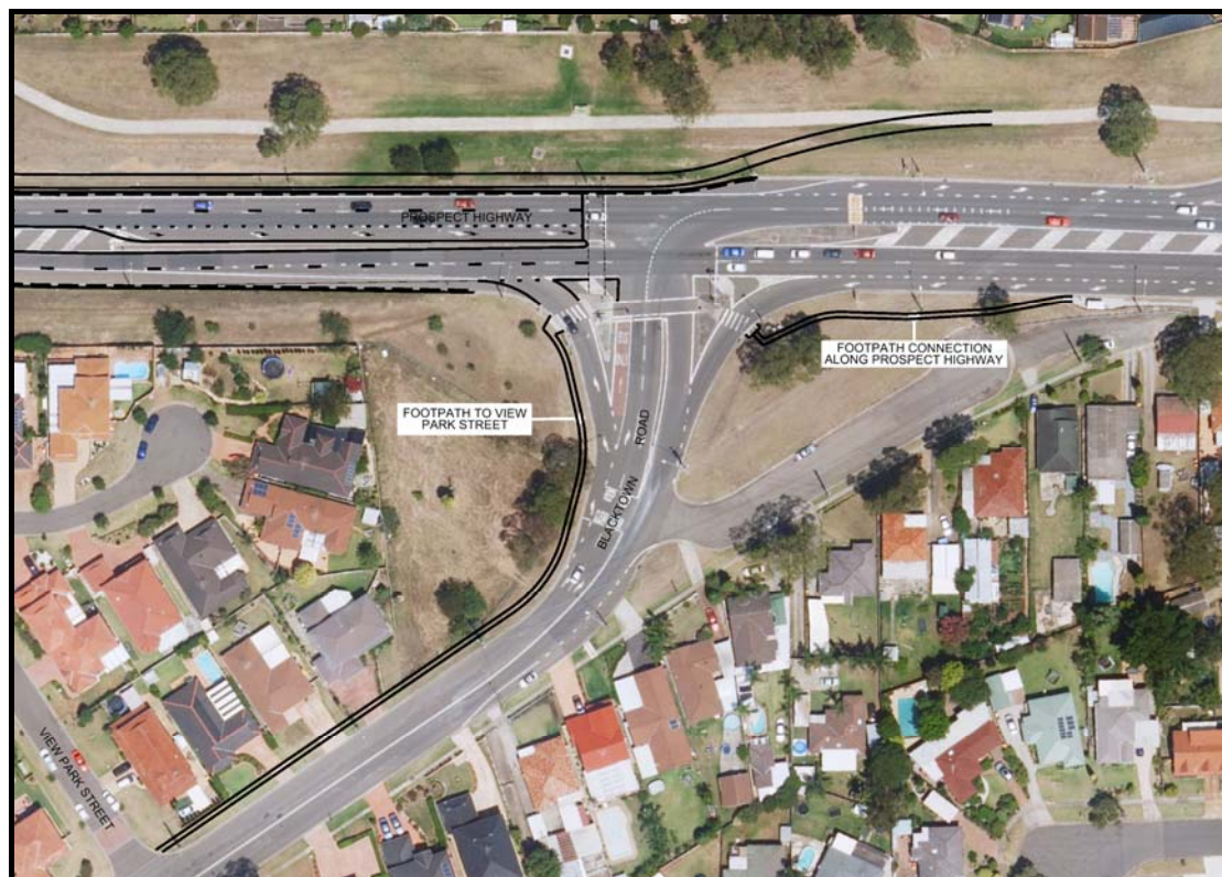
Figure 4-5 New footpath connections at Blacktown Road intersection
