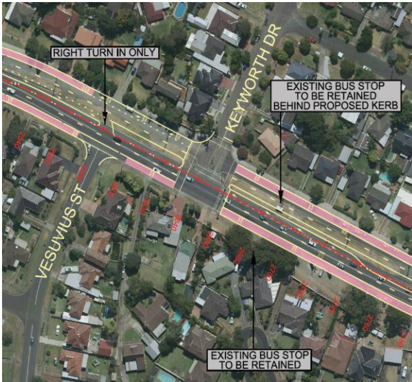
Figure 3.7: Provision of bus lanes on the approaches to Vesuvius Street and Keyworth Drive
