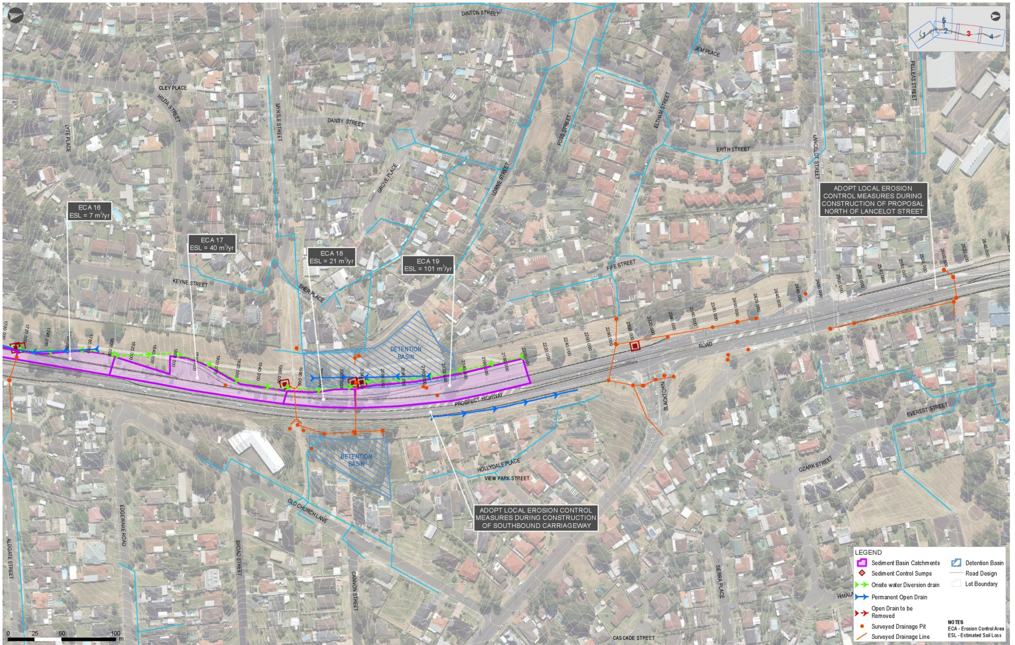
Figure 6-32 Construction erosion and sediment control 3
