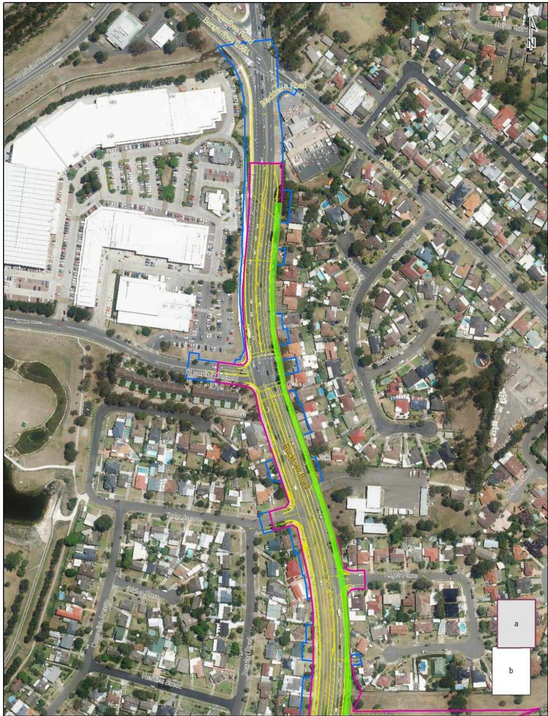
— REF approved project boundary — Proposed powerline relocation and clearing — Addendum REF project boundary Prospect Highway Upgrade 30012378 Powerline relocation between Bungarrabee Road and Blacktown Road Fig. 3-4a Aerial: © Land and Property Information 2015 0 50 100 Metres Last updated by: RC10721 on 15/06/2016 at 11:22 Location: I:\projects\30012378 - Prospect Highway Upgrade\008 DATA\GIS\Maps\Addendum REF\3-4 Proposed Powerline Relocation and Clearing.mxd
