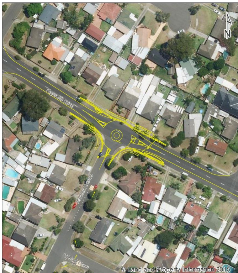
Figure 3-8 Roundabout at Hadrian Avenue and Keyworth Drive
