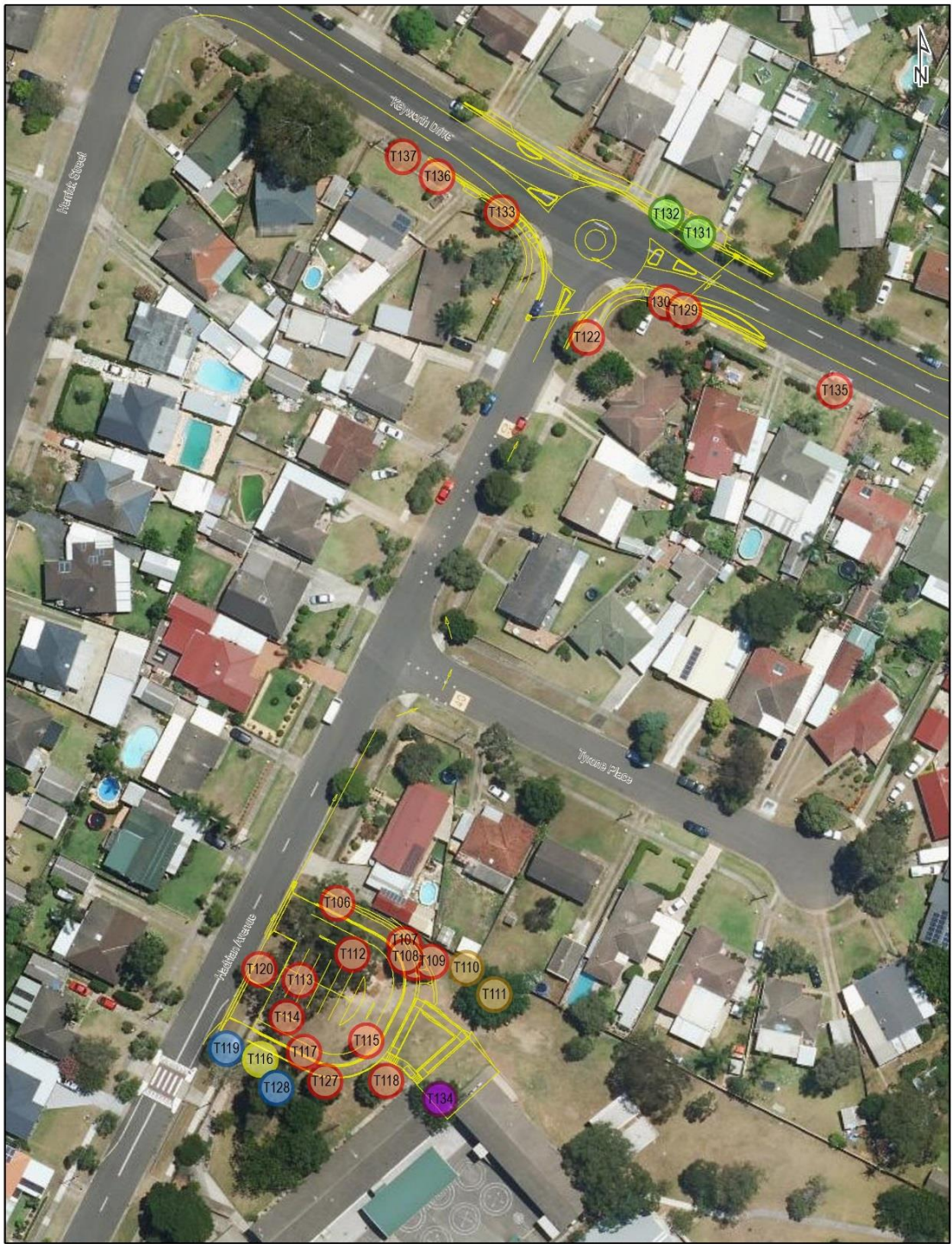
Prospect Highway Upgrade 30012378 Tree clearing required for kiss and ride facility and Hadrian Avenue roundabout & utilities relocation Fig. 6-6
