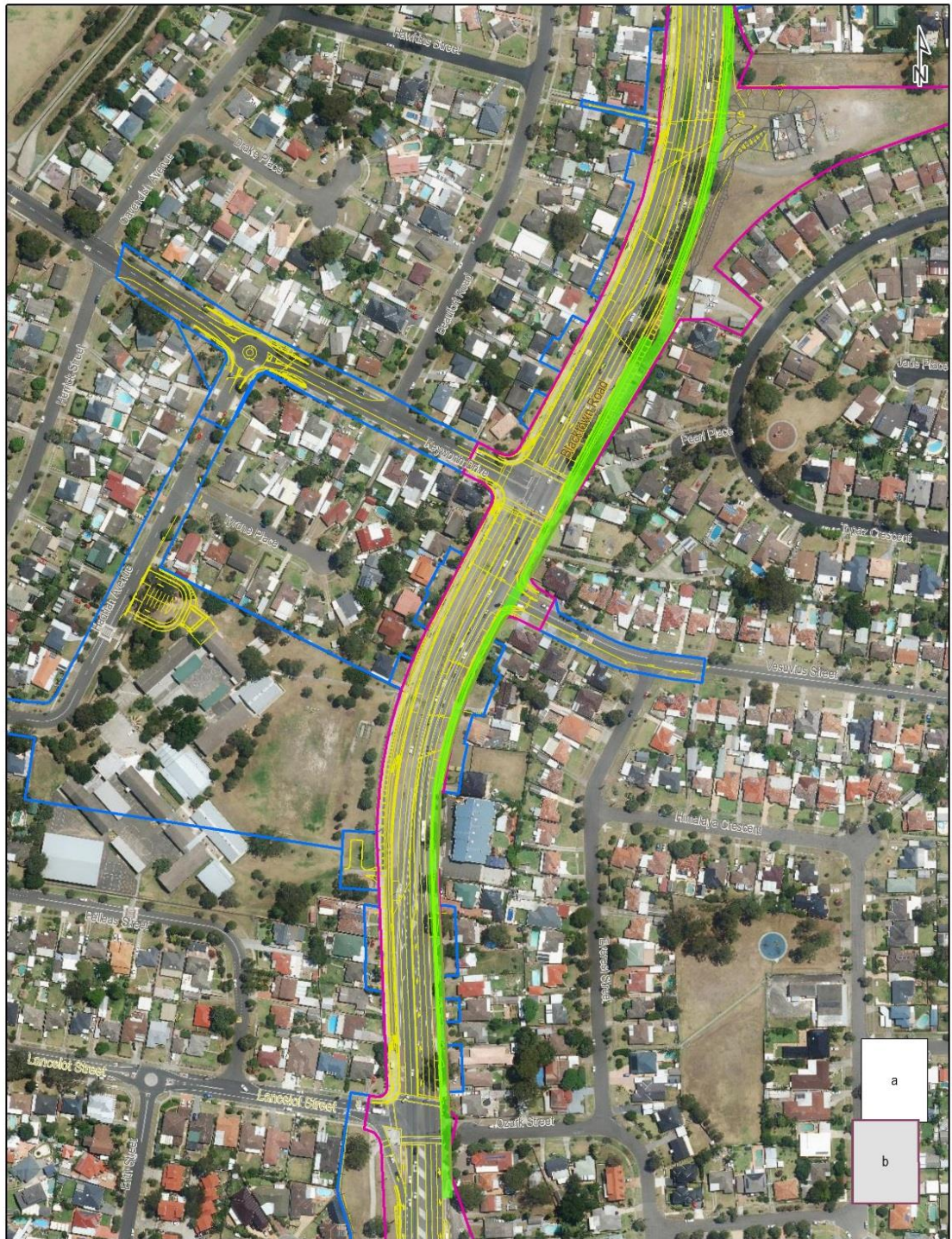
— REF approved project boundary — Proposed powerline relocation and clearing — Addendum REF project boundary Prospect Highway Upgrade 30012378 Powerline relocation between Bungarrabee Road and Blacktown Road Fig. 3-4b Aerial: © Land and Property Information 2015 0 50 100 Metres Last updated by: RC10721 on 18/08/2016 at 11:22 Location: I:\projects\30012378 - Prospect Highway Upgrade\008 DATA\GIS\Maps\Addendum REF\3-4 Proposed Powerline Relocation and Clearing.mxd
