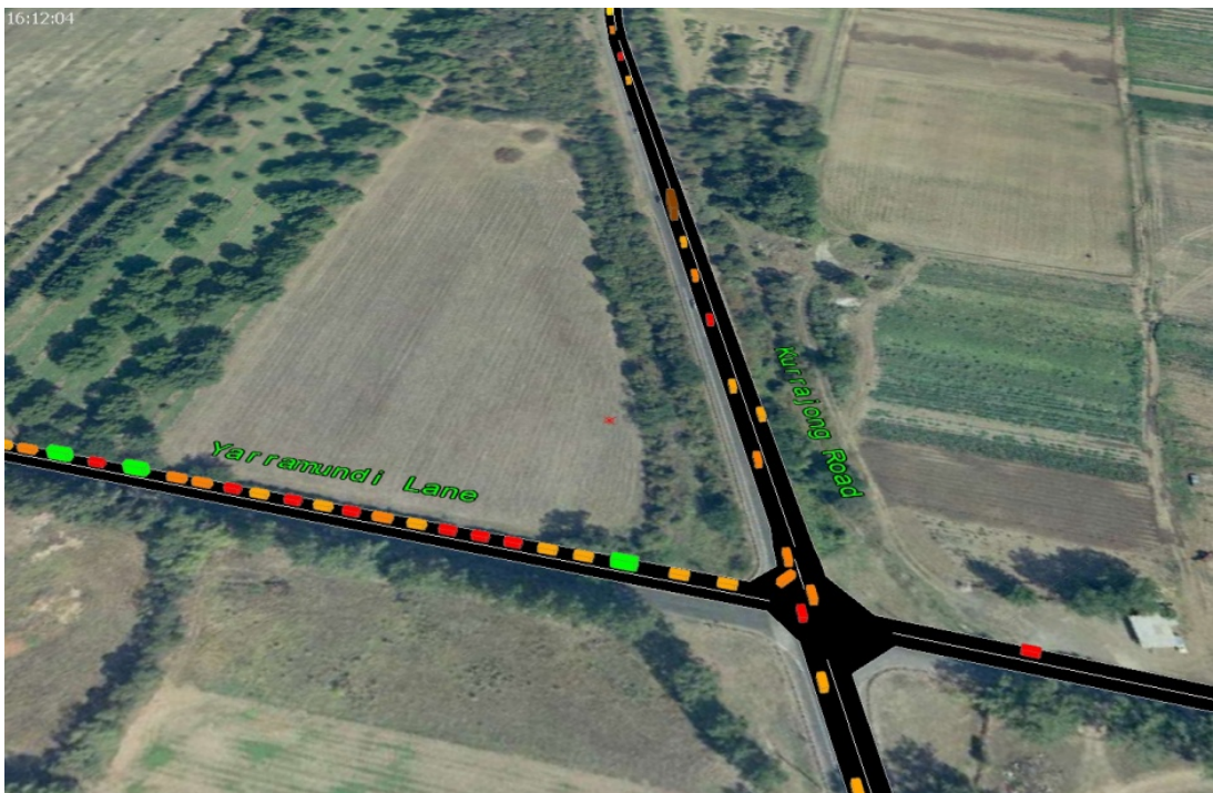
Figure 5-11 Kurrajong Rd/Yarramundi Lane intersection, westbound through traffic is frequently interrupted by aggressive left turning vehicles from Yarramundi Lane, PM peak;
