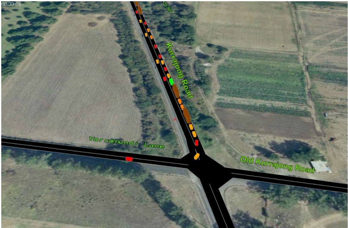
Figure 5-6 Right turn from Kurrajong Rd to Yarramundi Lane blocking eastbound through traffic, AM peak
