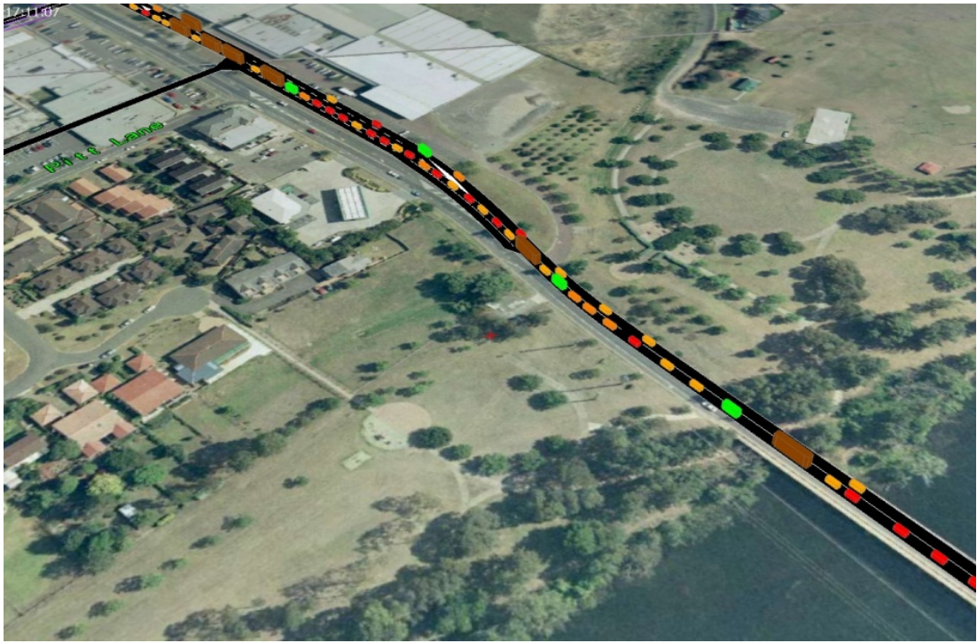
Figure 5-10 Bells Line of Road/Grose Vale Rd intersection, westbound queue is occasionally expanded to the bridge, PM Peak
