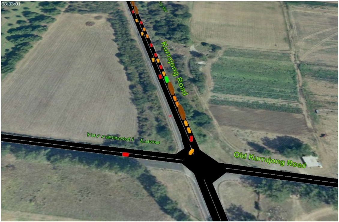
Figure 3-10 Right turn from Kurrajong Rd to Yarramundi Lane blocking eastbound through traffic, AM peak
