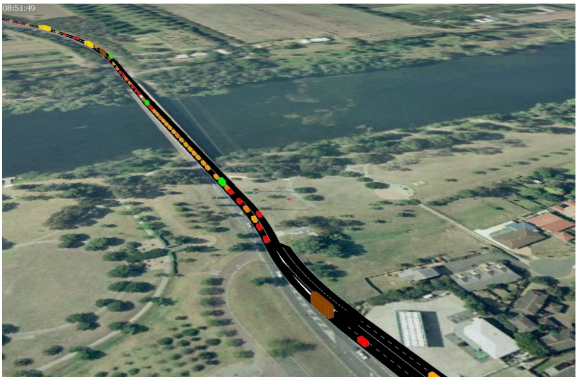
Figure 3-11 Eastbound traffic is occasionally stopped on the bridge due to downstream through traffic interruption at Yarramundi Lane, AM Peak
