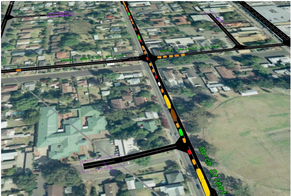
Figure 3-17 Typical PM peak westbound queue along March Street between East Market St and Bosworth St
