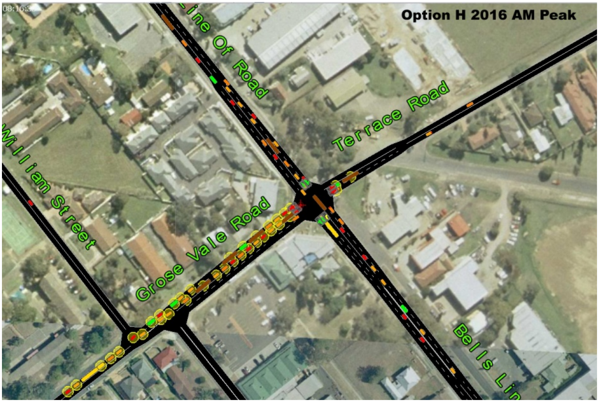
Figure D-13 2016 Option H AM Peak –Bells Line of Rd/Grose Vale Rd intersection
