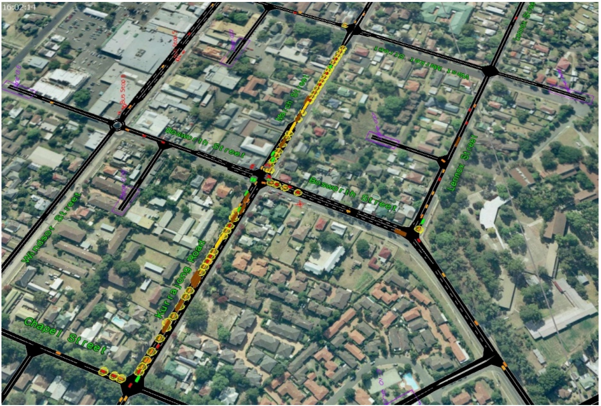
Figure D-16 2021 Option H PM Peak-Kurrajong Road/Bosworth St Intersection (with assumed clearway condition), showing expected queues along eastern (March St) and western (Kurrajong Rd) approaches
