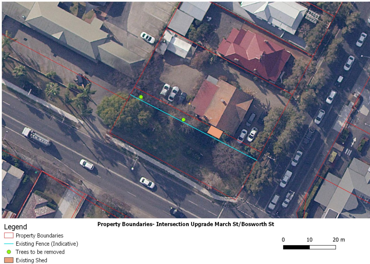
Figure 3-2 Location of shed and trees
