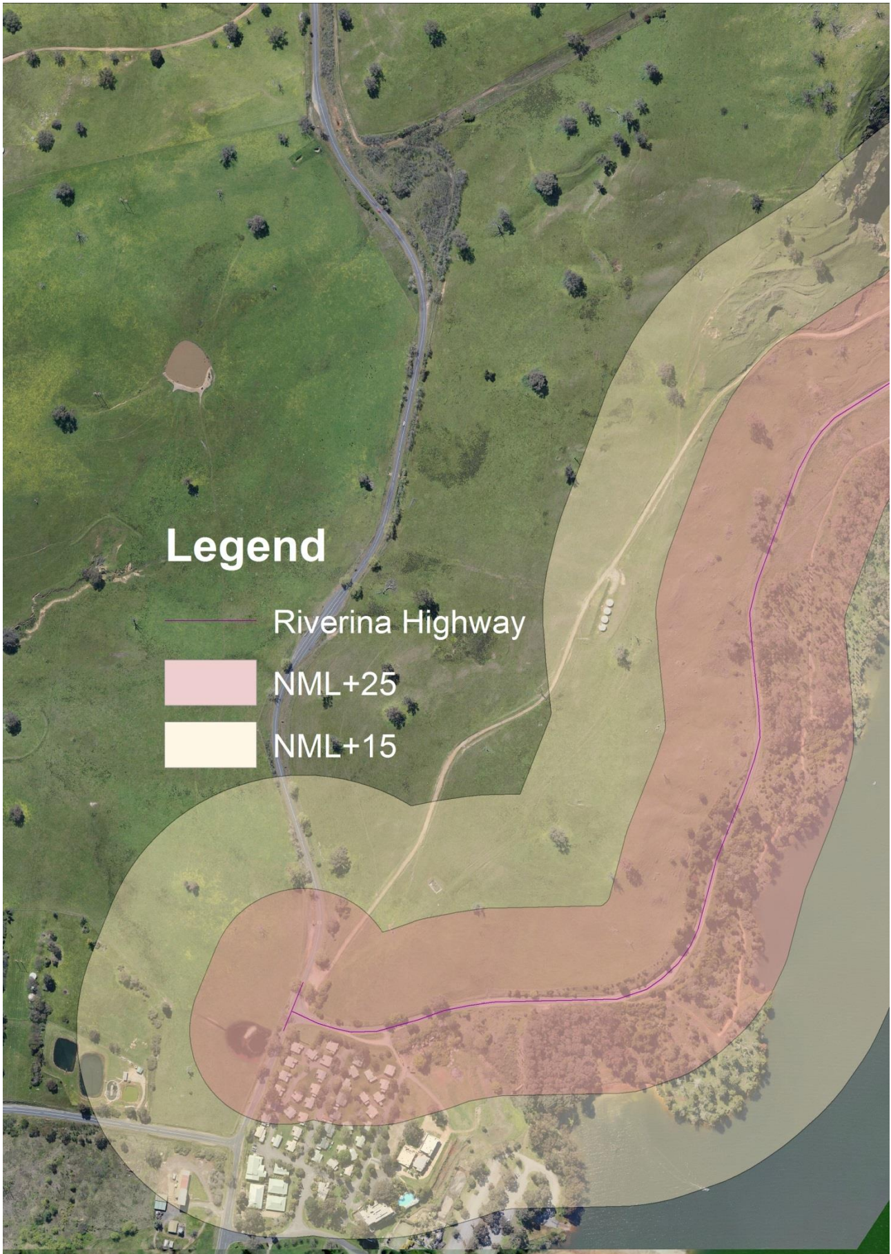
Sensitive receiver noise levels for bulk earthworks during daytime OOHW with no line of sight to the work. Source: Esri ArcGIS
