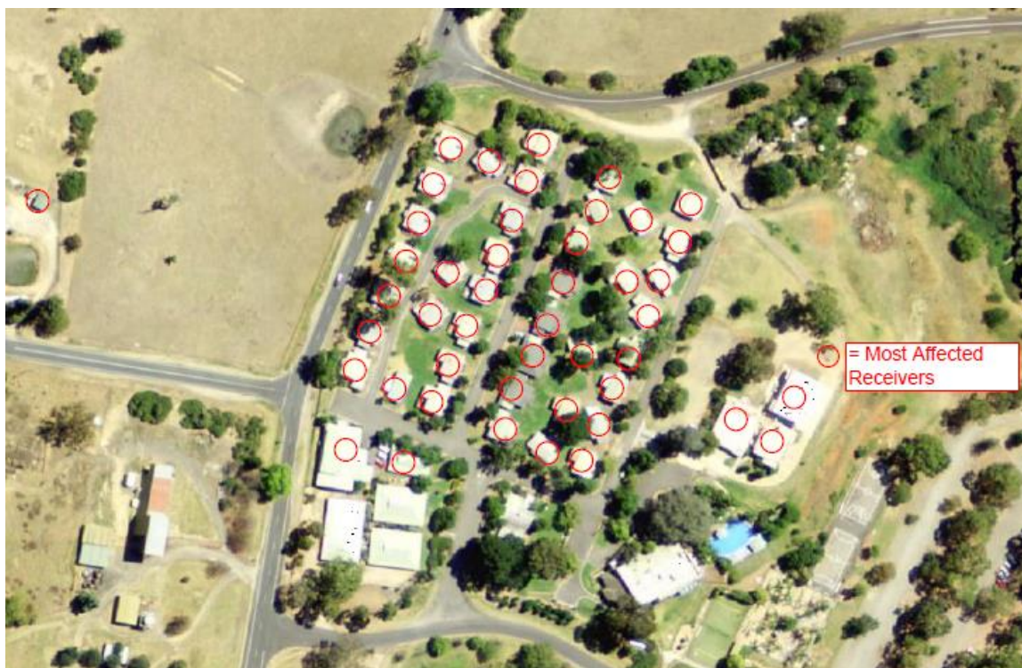
Figure 5) The most affected receivers during bulk earthworks are circled in red.
