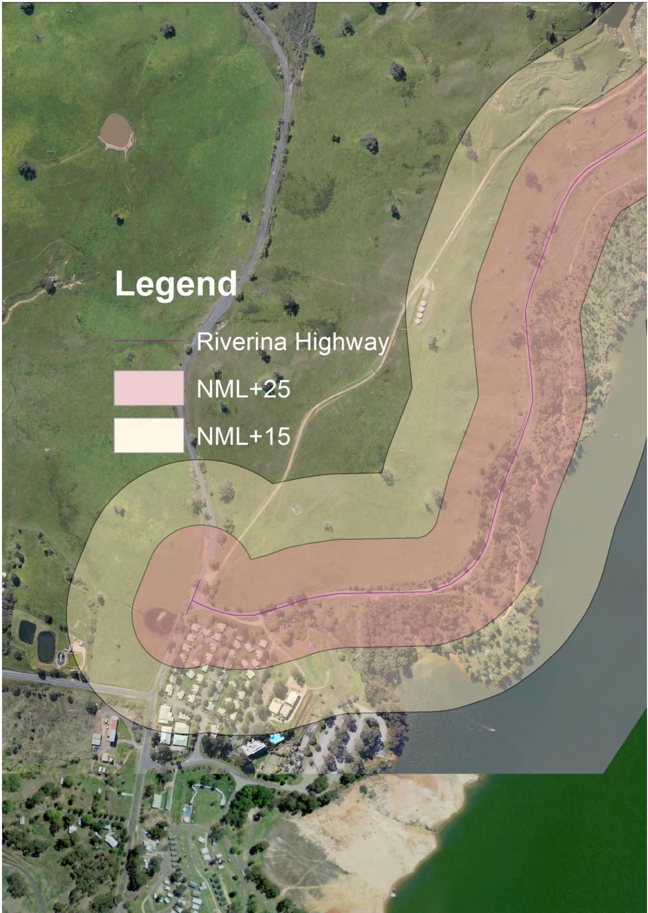
Sensitive receiver noise levels for road pavement construction during daytime OOHW with a line of sight to the work. Source: Esri ArcGIS
