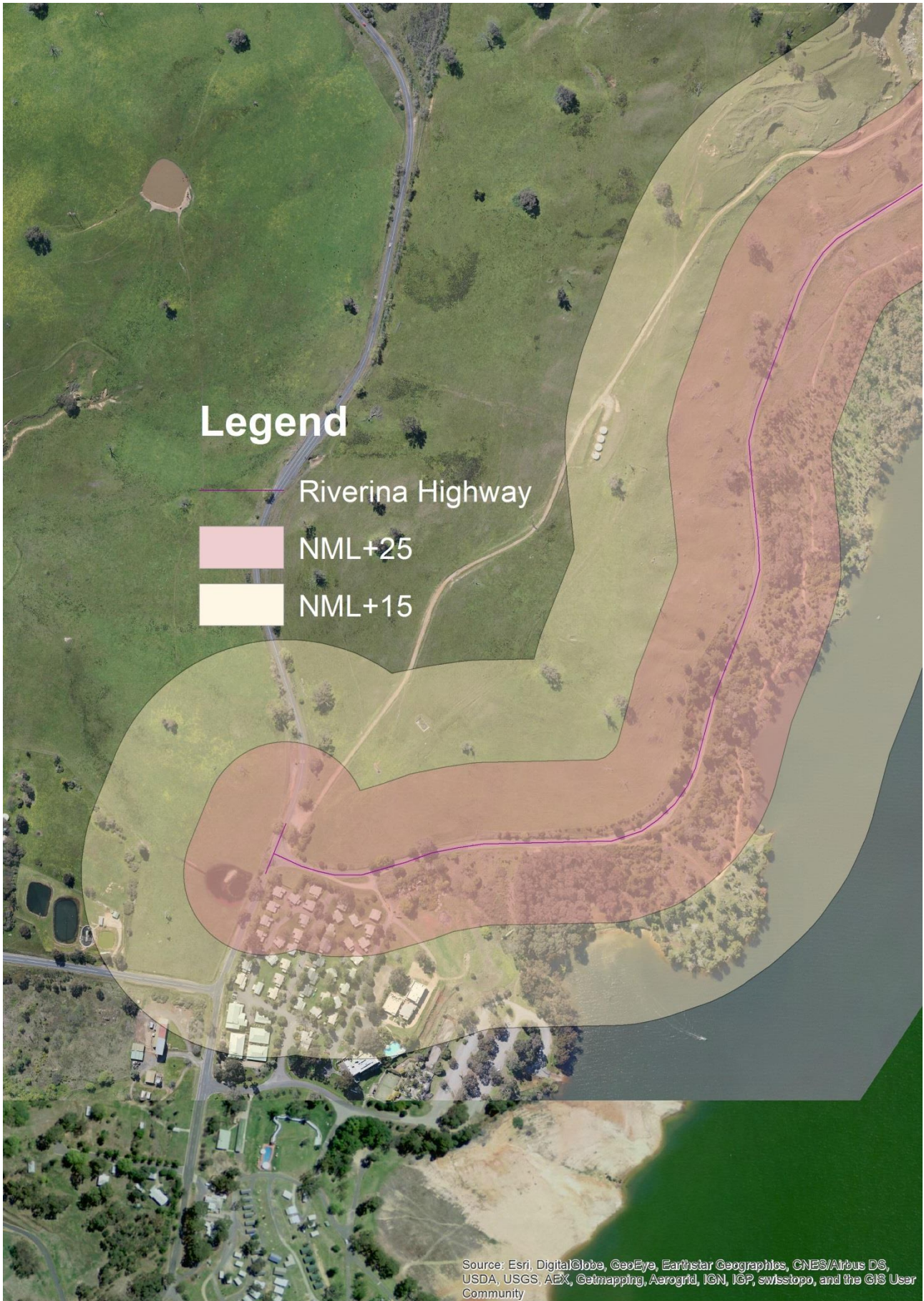
Sensitive receiver noise levels for corridor clearing activities during daytime OOHW with no line of sight to the work. Source: Esri ArcGIS
