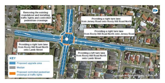
Image One: Proposed improvements to the intersection of Rooty Hill Road North, Jersey Road and Lamb Street, Plumpton
