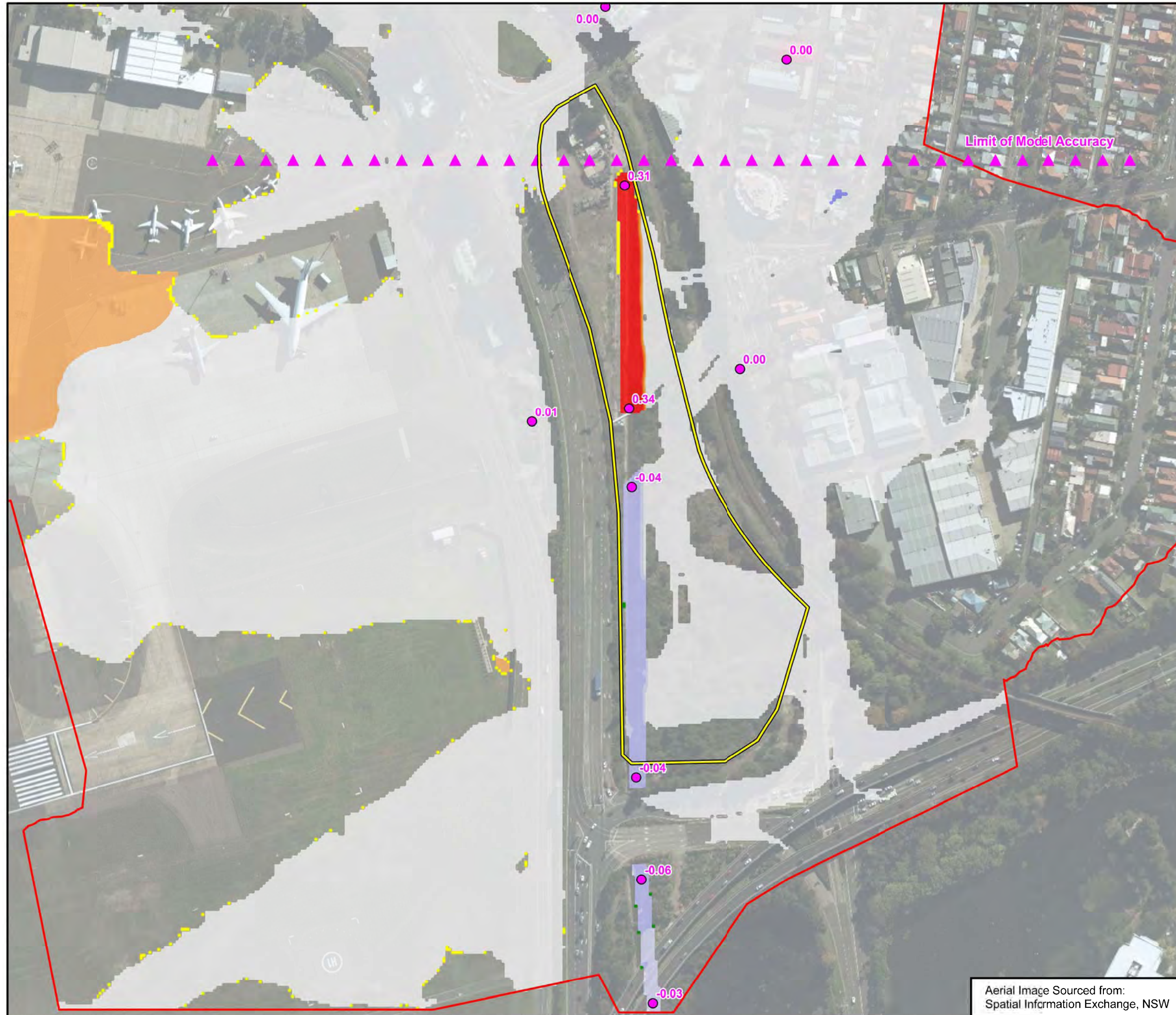
Figure 6.18 Airport East Precinct Works Flood Difference 1% AEP Sensitivity Assessment Culvert Option 1 50% Blockage Conditions
