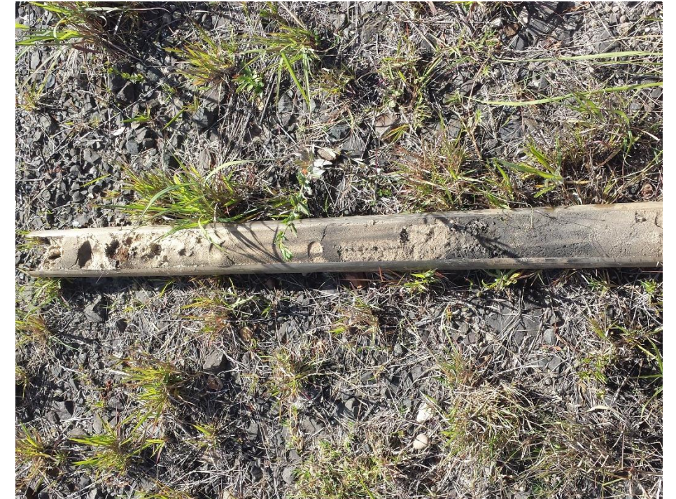
Photograph 3 – Sandy clay within the rail corridor (BH44/MW1 – 2.0 m)
