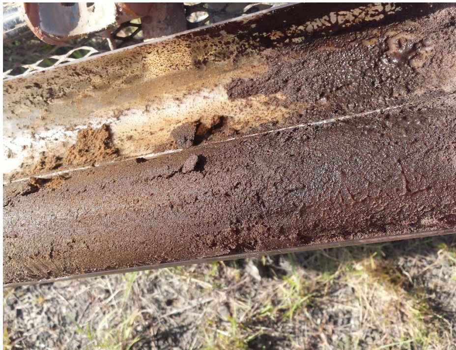
Photograph 4 – Water bearing zone within rail corridor (BH44/MW1 – 5.5 m)
