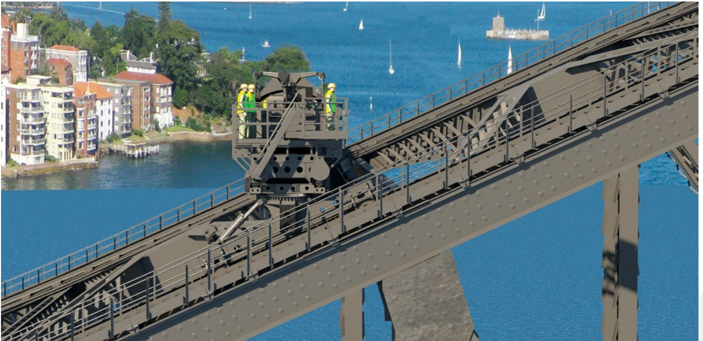
Artists impressions of one of the new arch maintenance units viewed from the side
