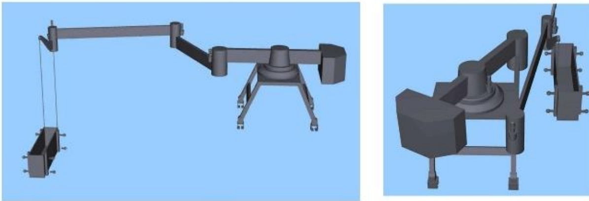
Figure 7 BMU Tender Design: Option 1: Knuckle JIB Images: ARUP
