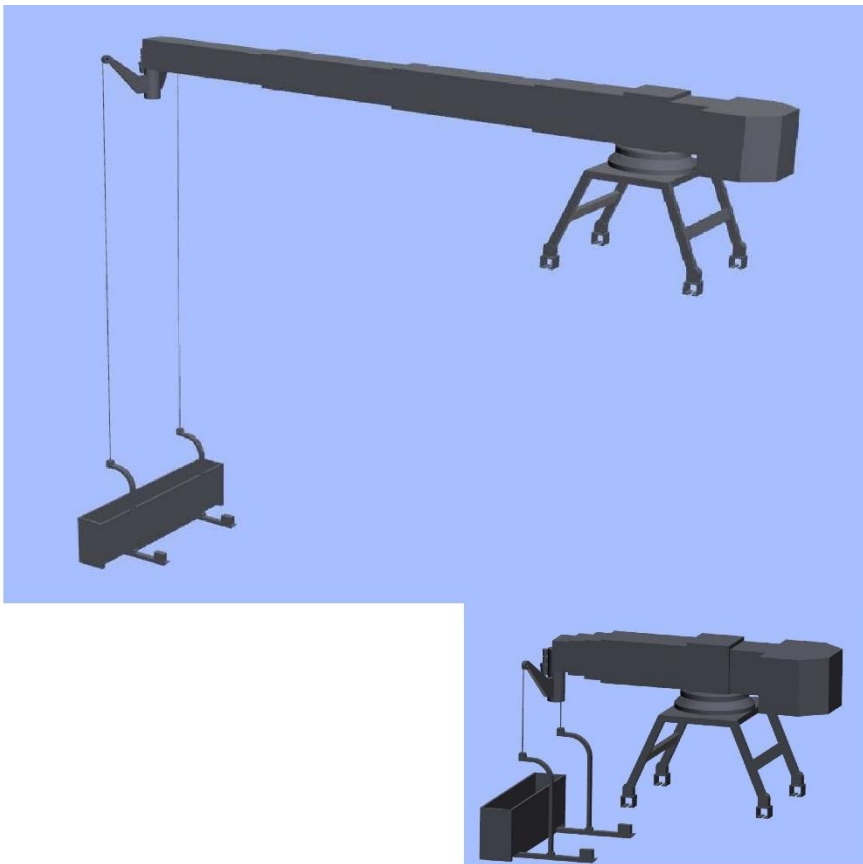
Figure 8 BMU Tender Design: Option 2: Telescopic JIB Images: ARUP
