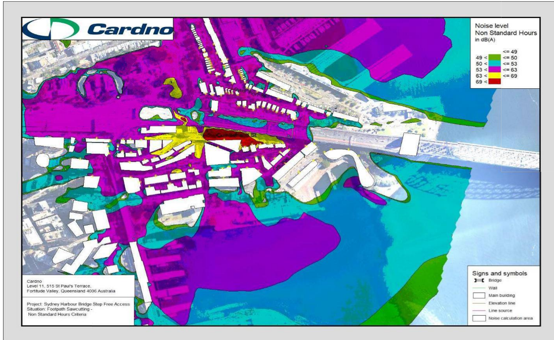
Figure 3: Scenario 1a (south) –Footpath Saw Cutting
