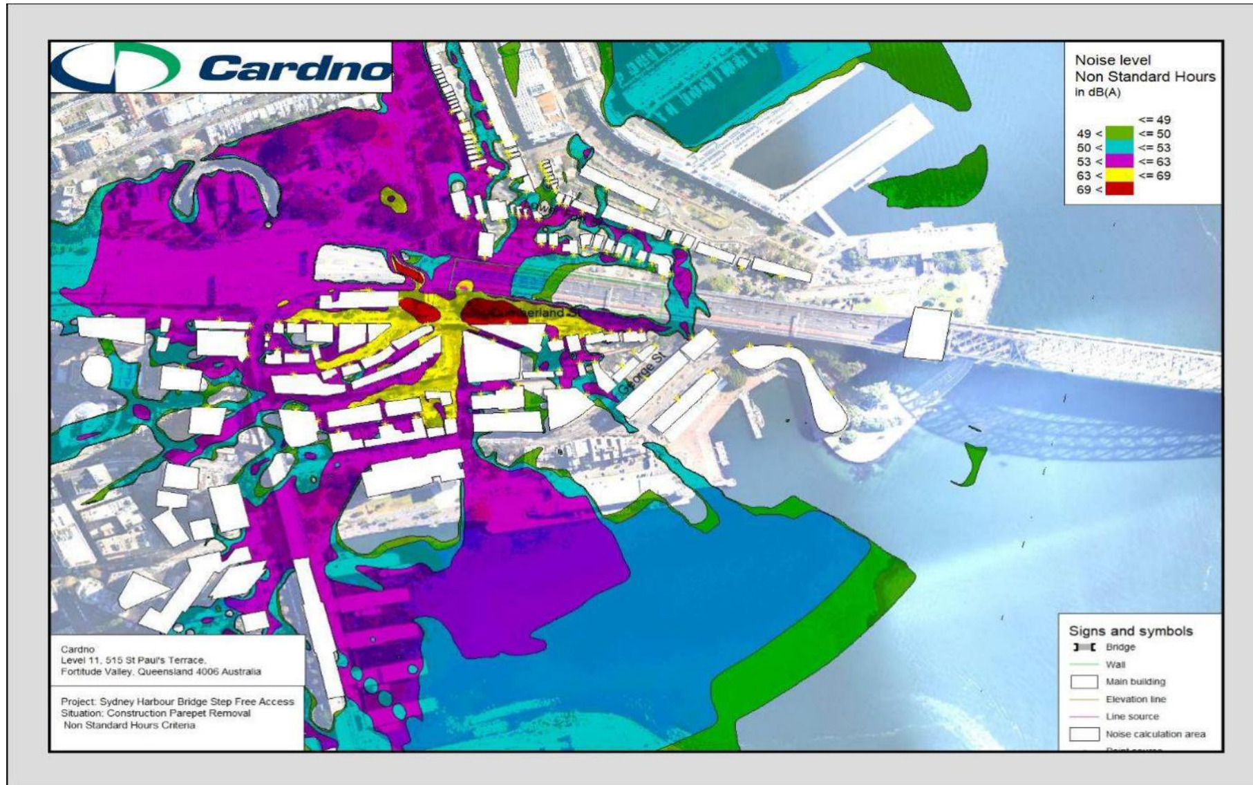
Figure 6: Scenario 2a (south) – Lift Construction (Parapet Removal)
